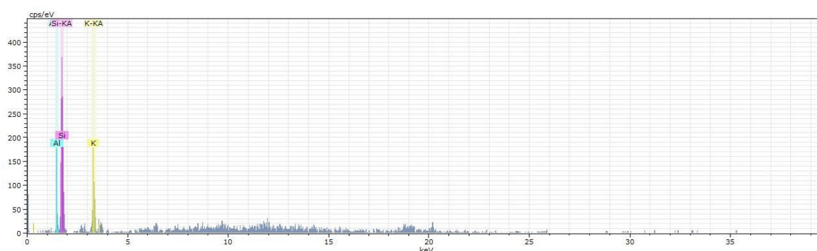
Figure 4-40: Spectrum of phases identified in Spot 3 (Aggregate)
