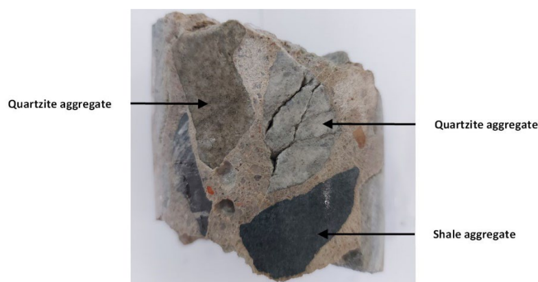
Figure 4-12: Image of a piece of Core 6B illustrating quartzite and shale coarse aggregates used in the construction of RC railway bridge
