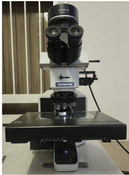
Figure 3-5: Olympus BX41 microscope with a digital Olympus DP74 camera attached
