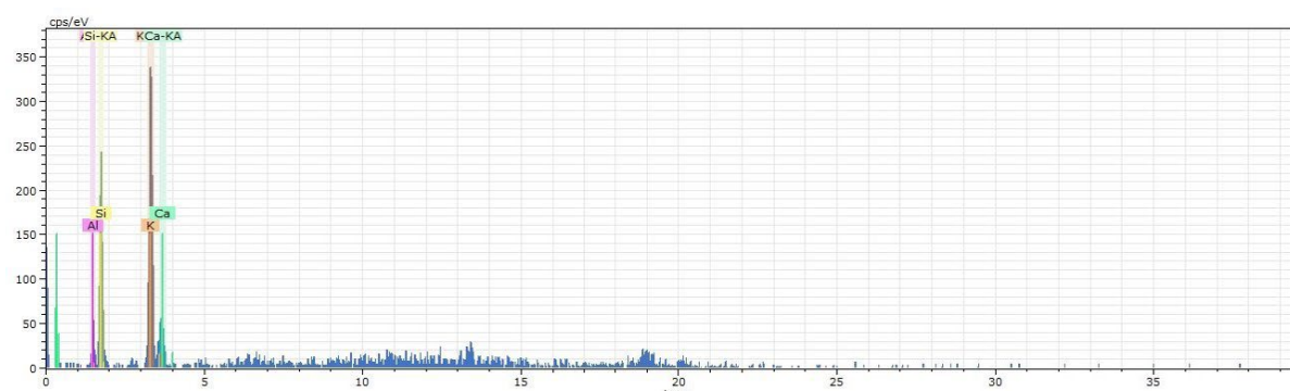
Figure 4-39: Spectrum of phases identified in Spot 2 (K-Rich Aggregate)
