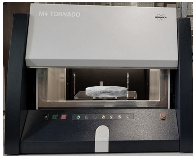
Figure 3-6: A flat concrete disc is placed on the Bruker M4 Tornado micro-XRF stage in preparation for the scan.
