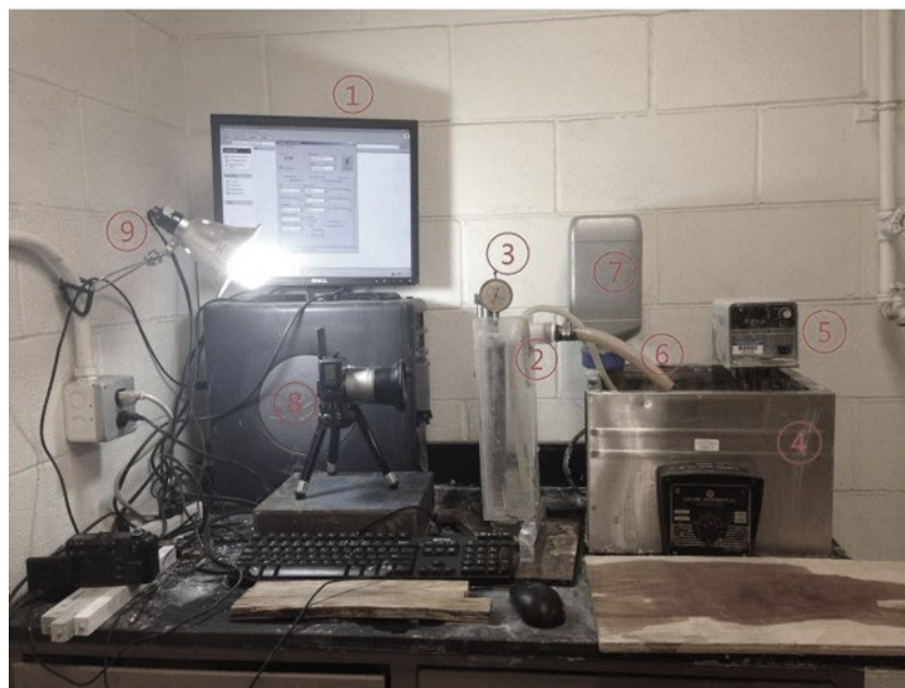
Figure 2-32: Experiment setup: 1-computer, 2-plexiglass container, 3-dial gauge, 4-reservoir, 5-immersion circulator, 6-tubing, 7-water drip bottle, 8-camera, and 9-lighting (Zhang, 2014)(Zhang, 2014)
