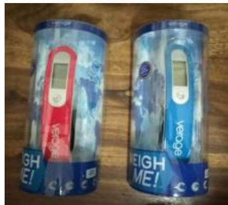
Figure 3.4 Travel hanging scales used to weigh manually handled loads
