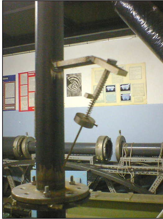
Figure 5.4. Photograph of the diaphragm bursting mechanism on “Mach 2” shock tube.
