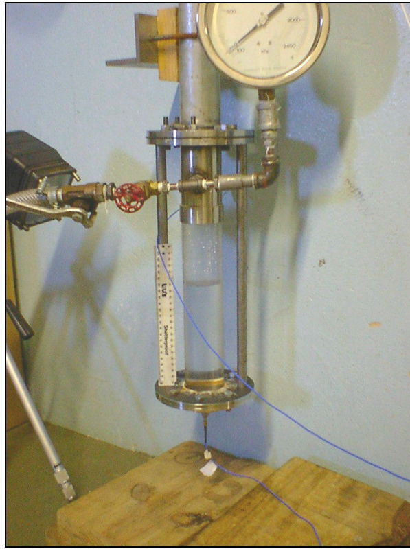
Figure 5.2. Photograph of the “Mach 3” shock tube test (driver) section.
