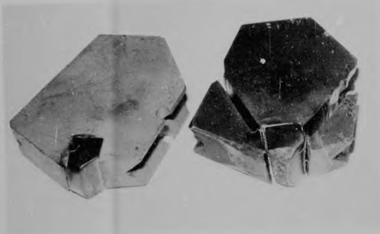
FIGURE 14. Rockcutter bit, showing method of breaking open to examine the braze joint.
