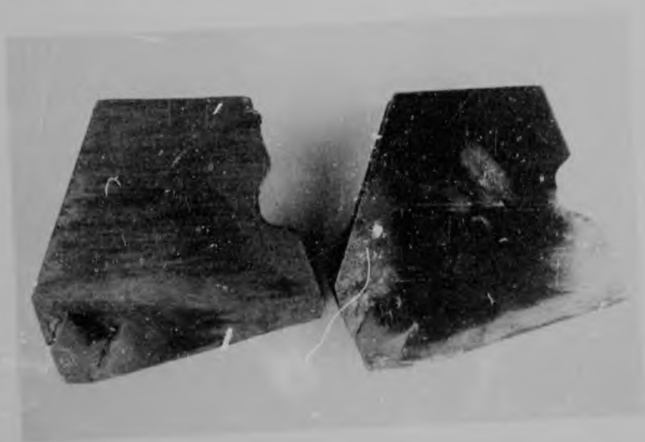
FIGURE 76. Photograph showing wear of steel bit body when a water jet was not used.
