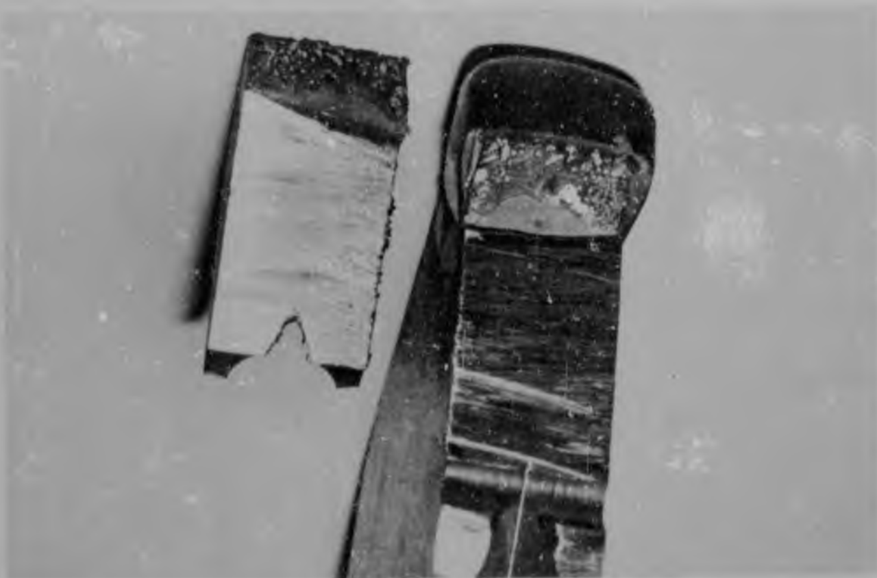
FIGURE 15. Oxidation of front braze face.
