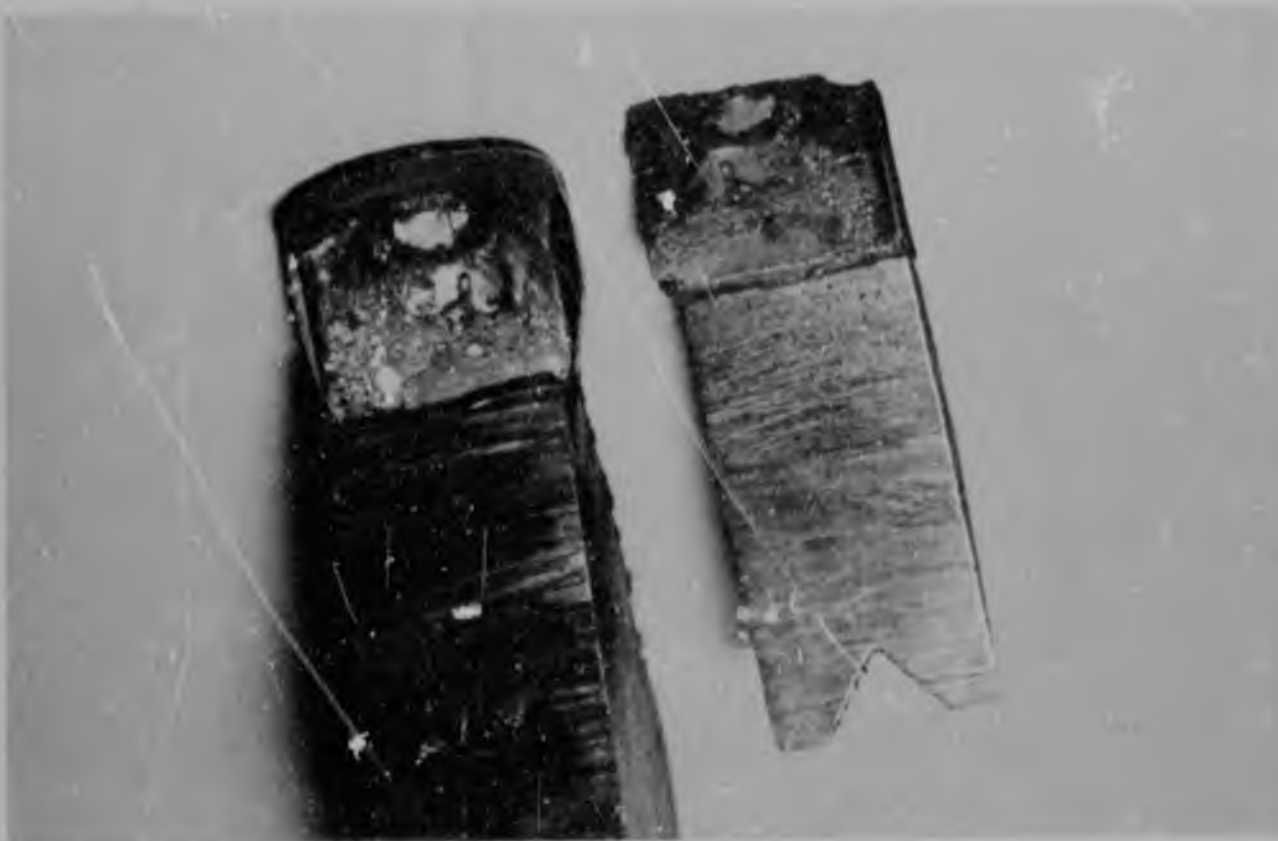
FIGURE 16. Oxidation of rear braze face.
