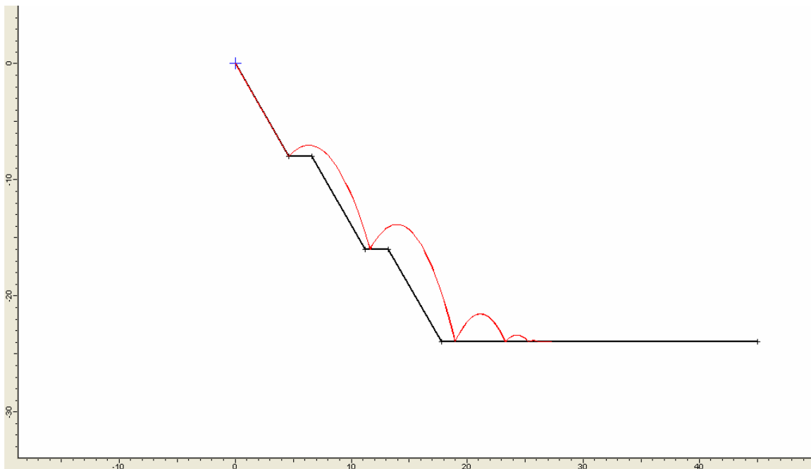
Figure A7. Rockfall paths of rock type One at horizontal velocity of 0.1 m/s with standard deviation of 0.01.
