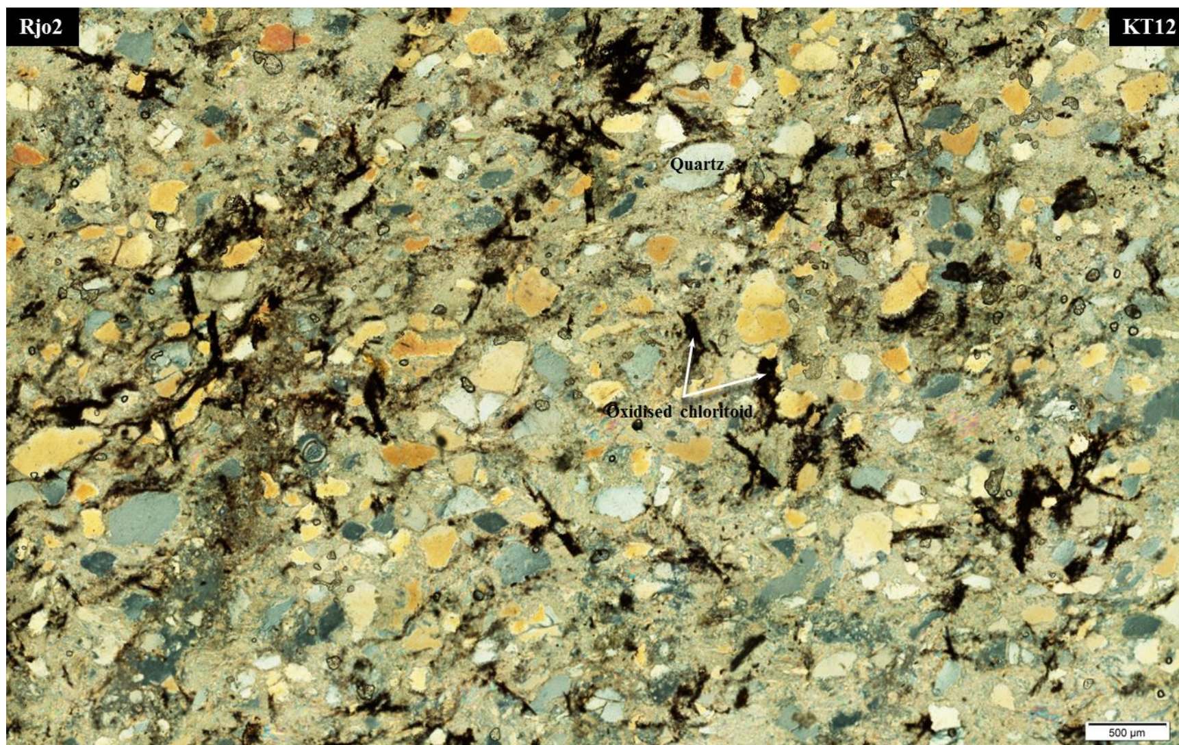
Figure 4.11. Photomicrograph mosaic of the KT12 knotted quartzite sample. The sample is composed of 38% quartz, 47% sericite+muscovite, 13% chloritoid, 2% rutile+zircon (DIC).
