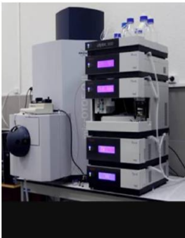
Figure 70: Ultra-High-Performance Liquid Chromatography (Thermo Scientific Ultimate 3000, RS diodearray detectors) with a Diode Array (190, 195, 215, 254, and 300 nm) coupled to a Bruker Compact QTOF high-resolution mass spectrometer.
