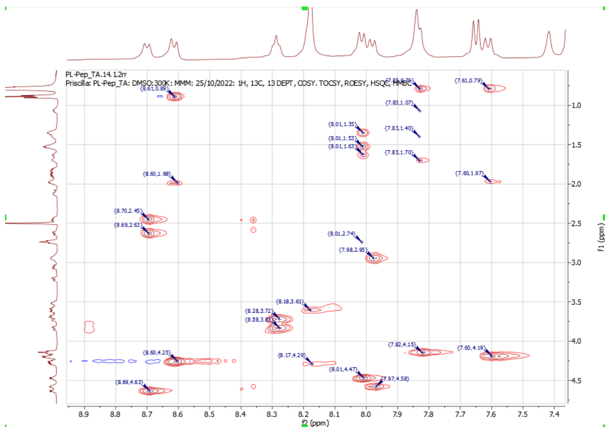
Figure 69: The TOCSY and COSY spectrums showing the fingerprint region.
