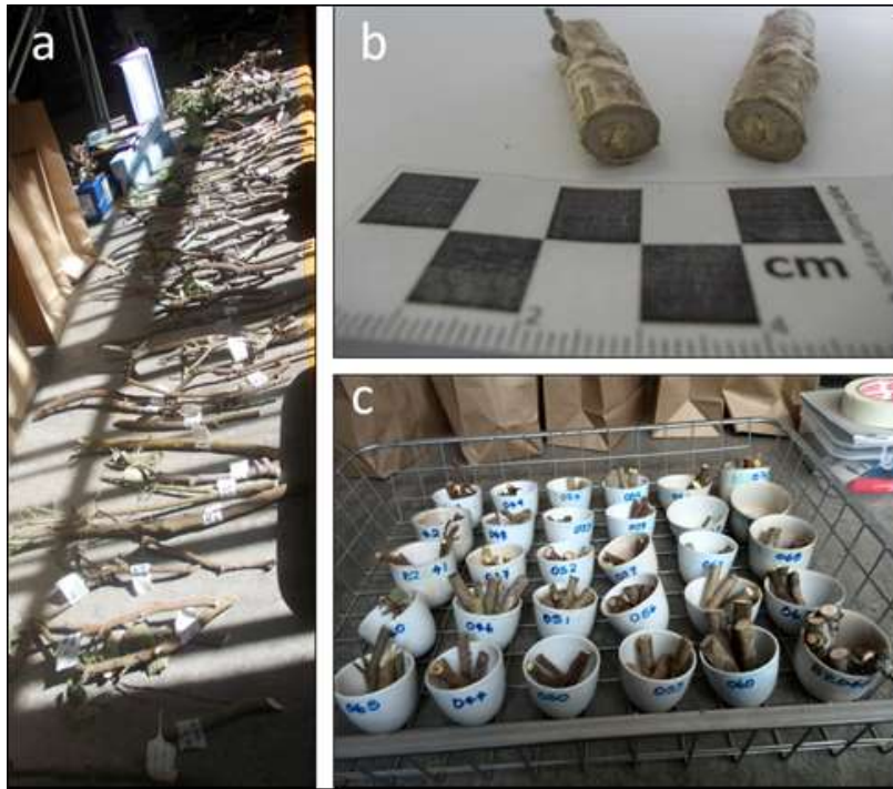
FIG. 3.2 The laboratory preparation of wood pieces. Wood pieces were (a) sun-dried, then (b) cut into smaller pieces and (c) loaded inside crucibles and desiccated in an oven.
