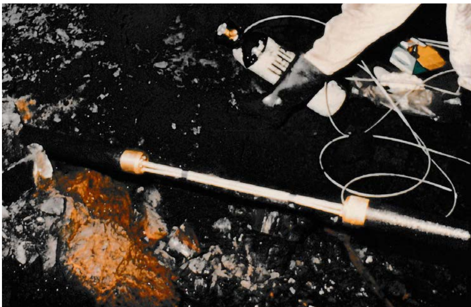
Figure 6.16 Installation of the packer in borehole (Source: Stripp, 1989)
