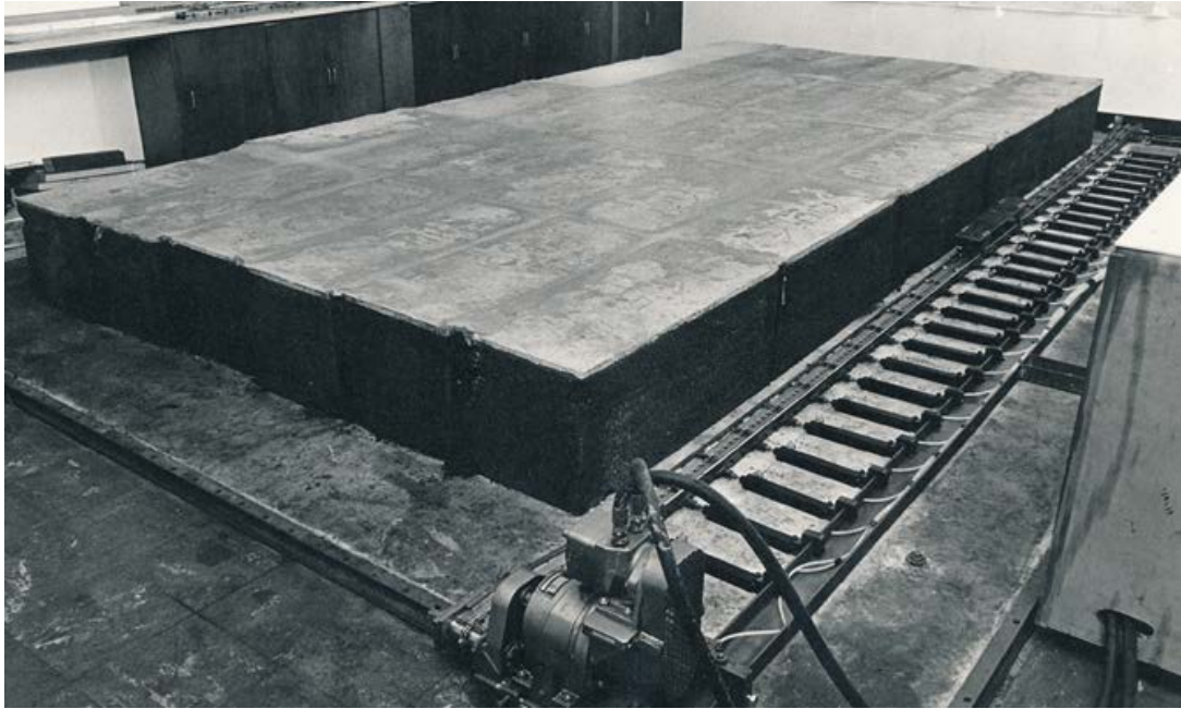
Figure 1.2 View of the \frac{1}{8} scale face, pushing rams and conveyor
