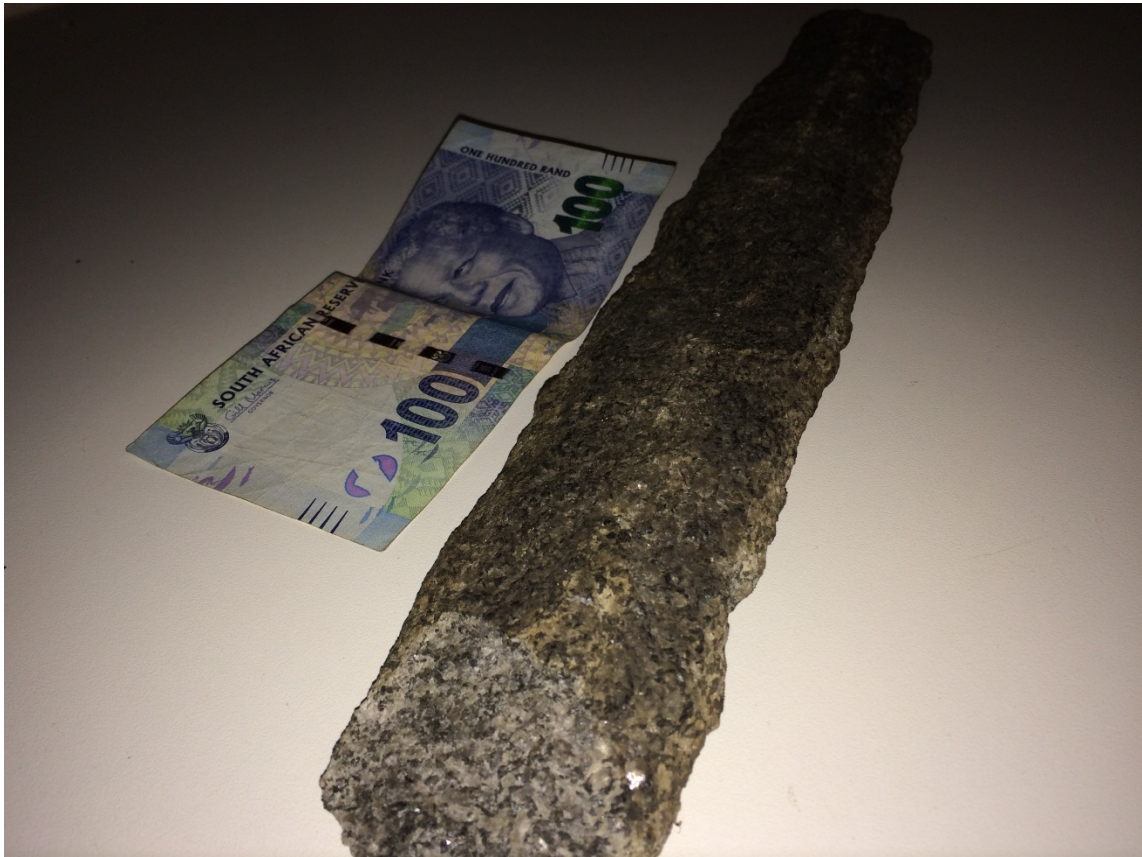
Figure 2.33 Slabbing between adjacent discs cutting South African Norite
