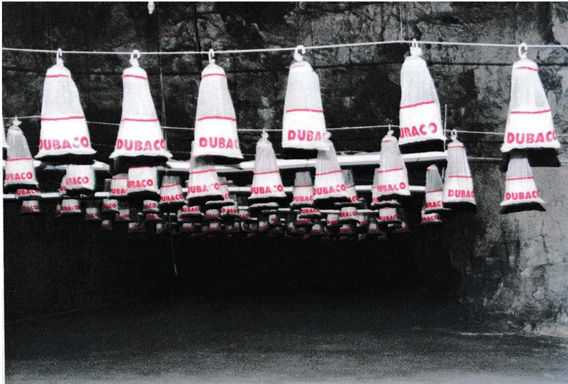
Figure 6.35 Bagged barrier installed for testing at Lake Lynn (Source: Du Plessis, 2000)
