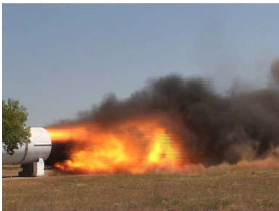
Figure 6.11 Unsuppressed coal dust explosion (Courtesy of Mr Isaac Mthombeni)
