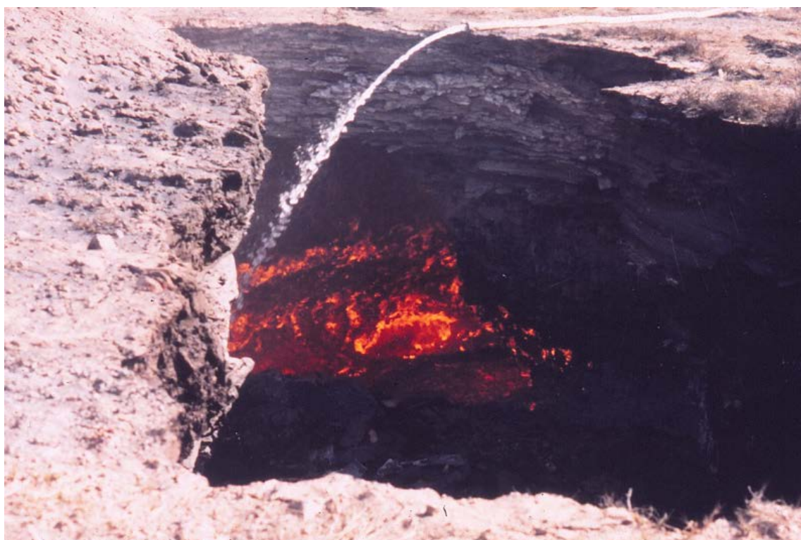
Figure 3.11 Full collapse of an intersection and an attempt to control an underground fire using water (Photograph taken by Phillips)
