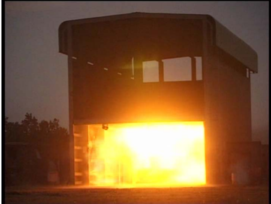
Figure 6.27 Unsuppressed methane explosion in empty 20m tunnel (Courtesy of Mr Isaac Mthombeni)
