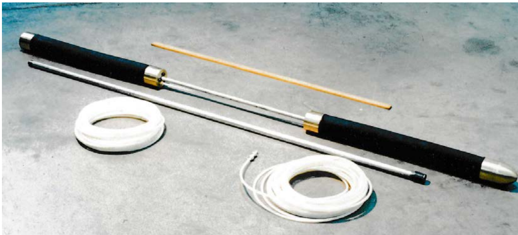
Figure 6.15 Complete packer assembly (Source: Stripp, 1989)
