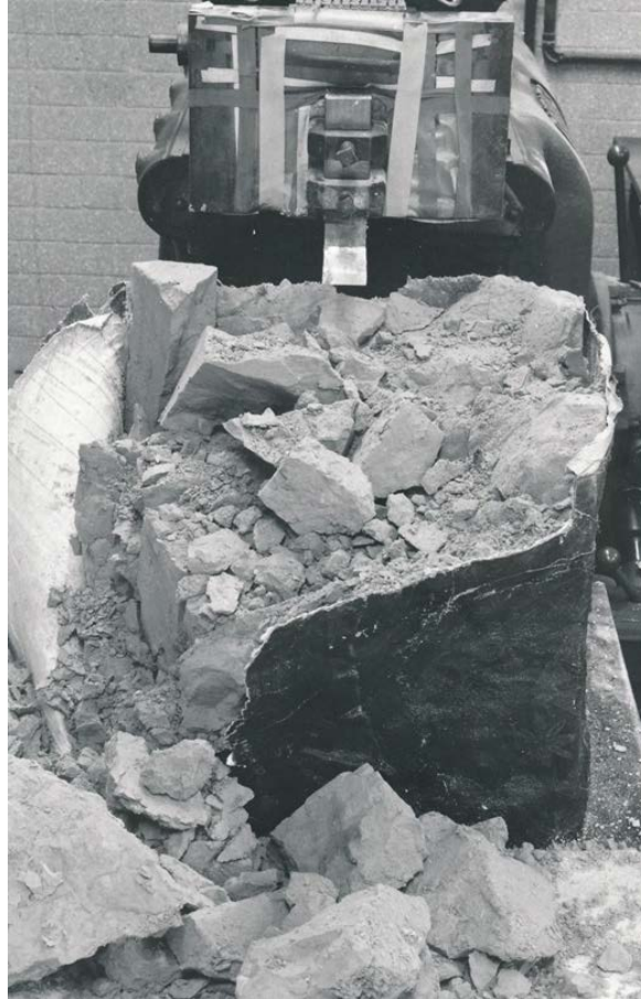
Figure 2.6 Collapse of a Lower Chalk sample (Source: Roxborough and Rispin, 1972)
