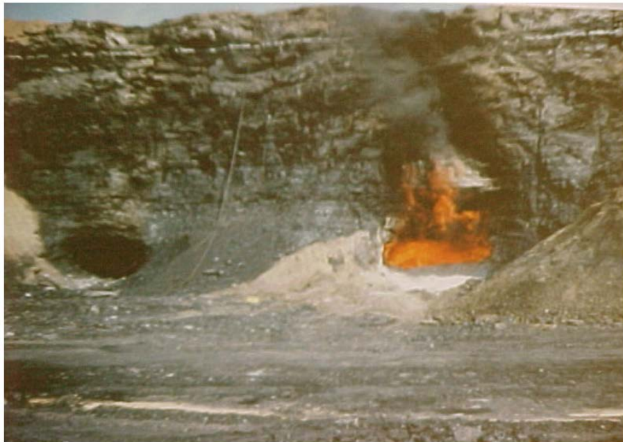
Figure 3.16 Surface mining of old bord and pillar workings
