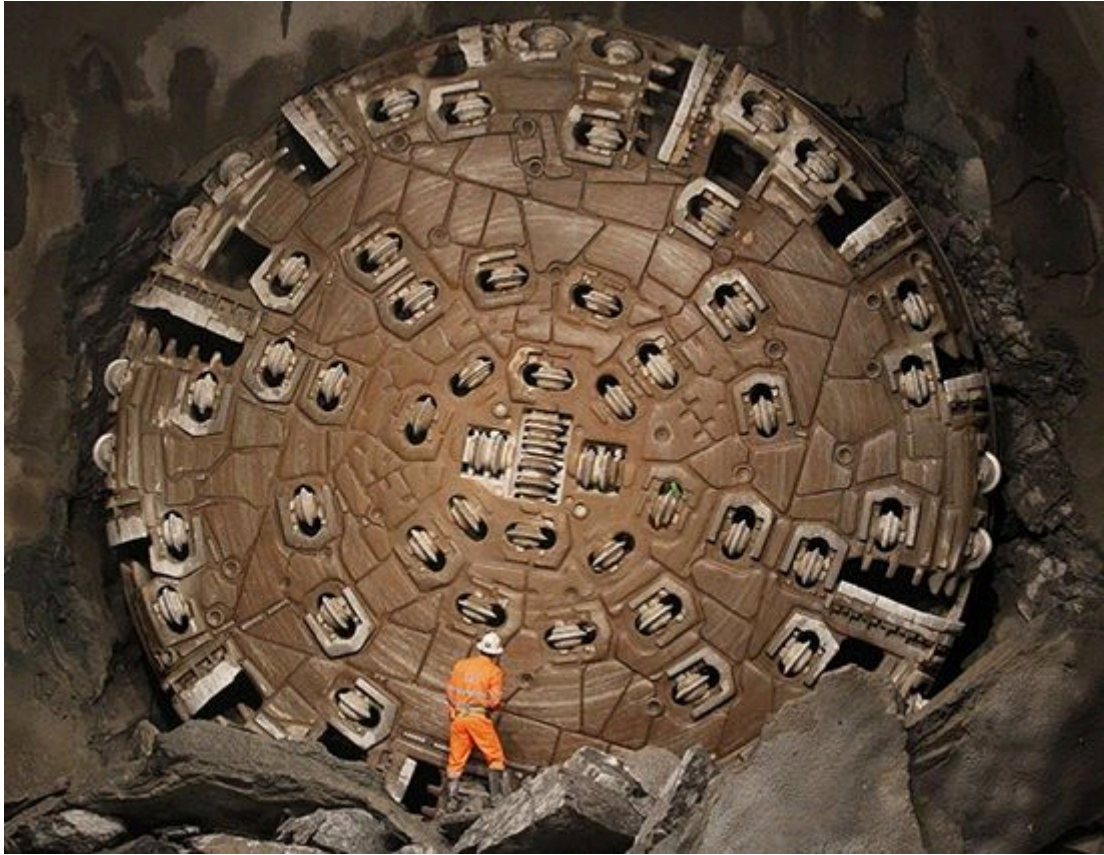
Figure 2.5 Disc cutters disposed on the head of a tunnel boring machine
