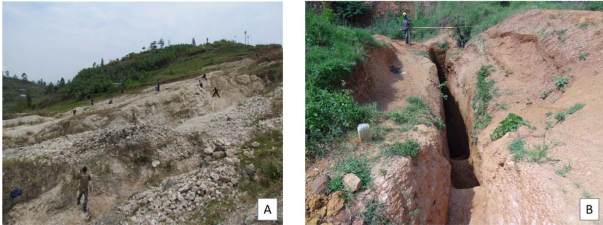
Figure 1. 7: Illustrations of (A) artisanal miners at Gatumba extracting minerals from secondary mineralisation whereas (B) is an old entrance to an abandoned underground mine extracting minerals from primary mineralisation (Montjoie, 2014; Muchez et al., 2014).
