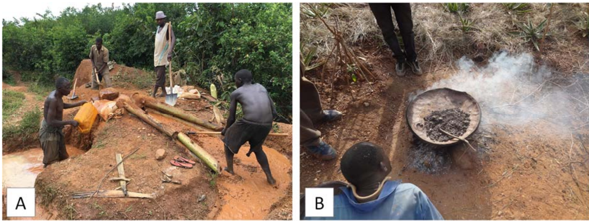
Figure 3.3: Artisanal miners on the HMR project, A) processing the ROM and B) drying the concentrate, using traditional methods.
