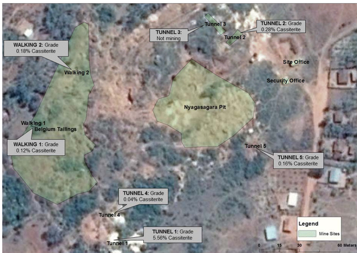
Figure 4. 2: Map of Nyagasagara, illustrating the locations and cassiterite grade of the various mining sites on the deposit; the Belgium miners used the Nyagasagara pit and Belgium tailings in the 1950s. The current mining areas are Tunnel 1 to 5.
