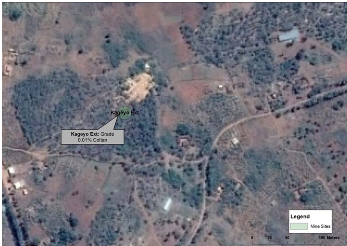
Figure 4. 7: Map of Kageyo Extension, illustrating the location and coltan grade observed at the mining sites.
