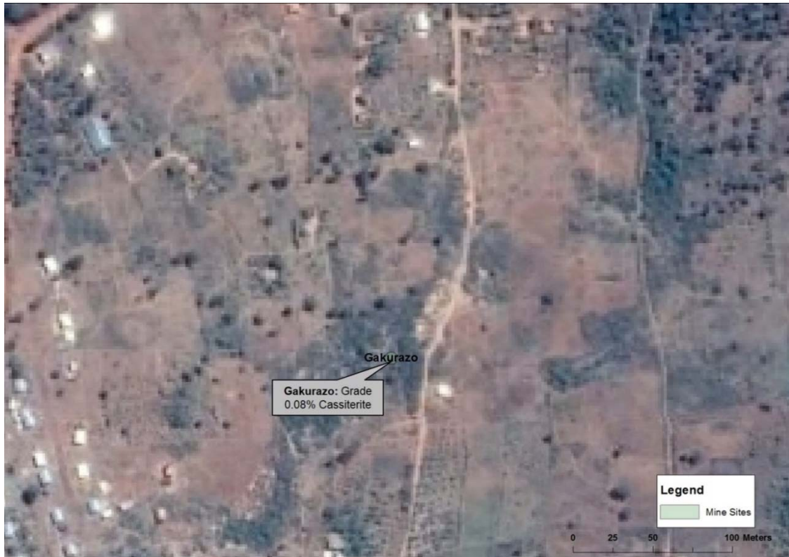
Figure 4. 4: Map of Gakurazo, illustrating the location and cassiterite grade of the mining site.
