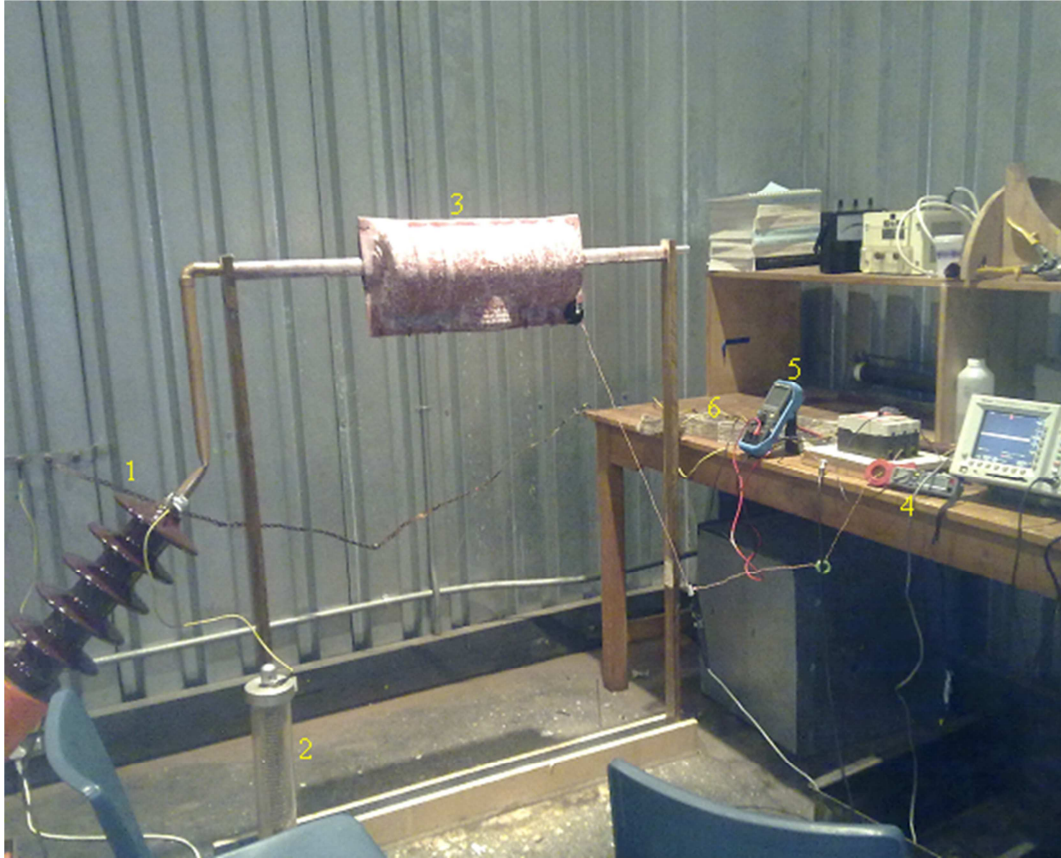
Figure 5-1: Experimental Set-up:1. HV bushing step up transformer, 2. Voltage divider, 3. Polluted insulated conductor cover, 4. Leakage current meter, 5. Multimeter, 6. Series resistance
