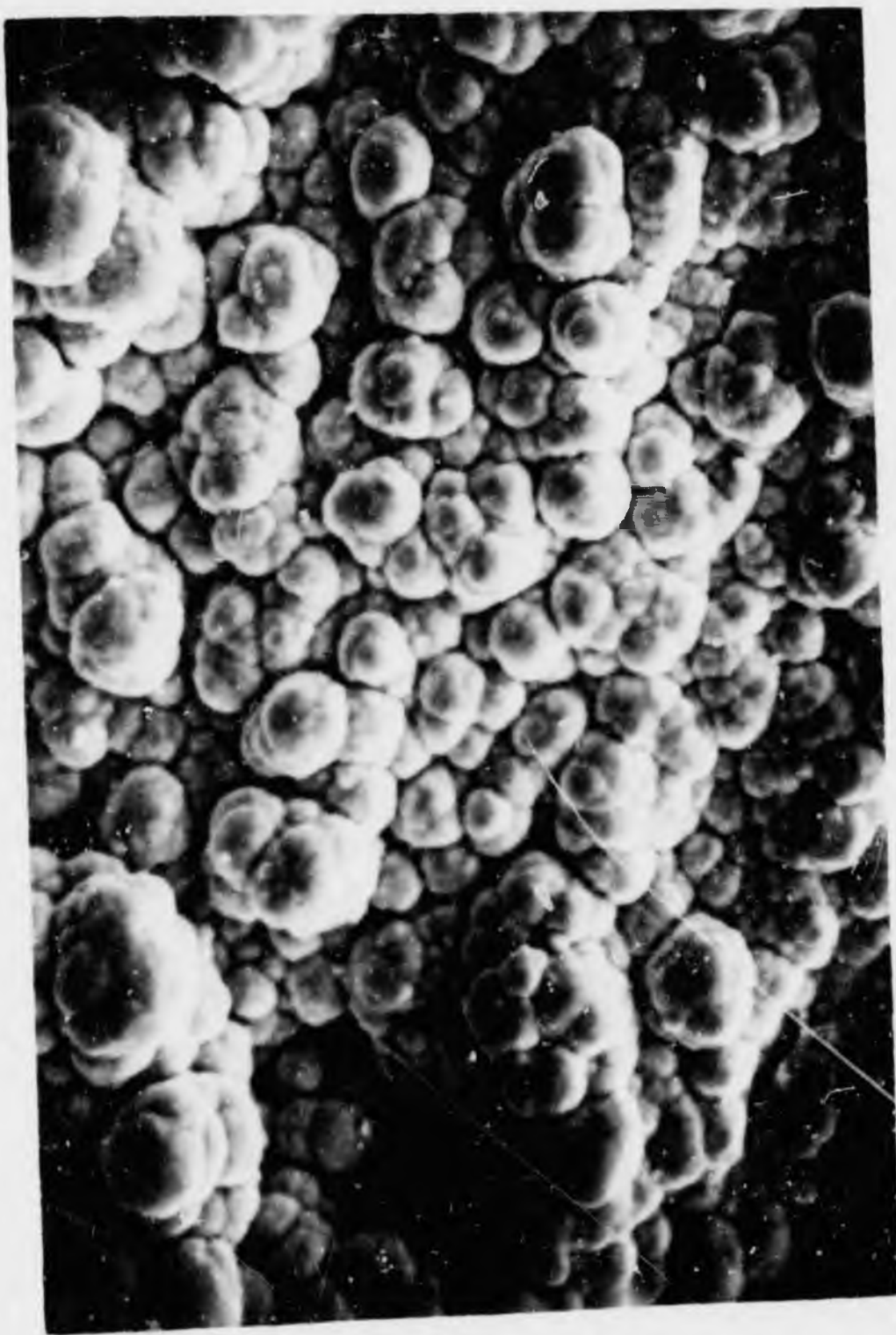
Plate 581112: Run 9 The roughest coat deposited on these particles. (Mag. 1200X)
