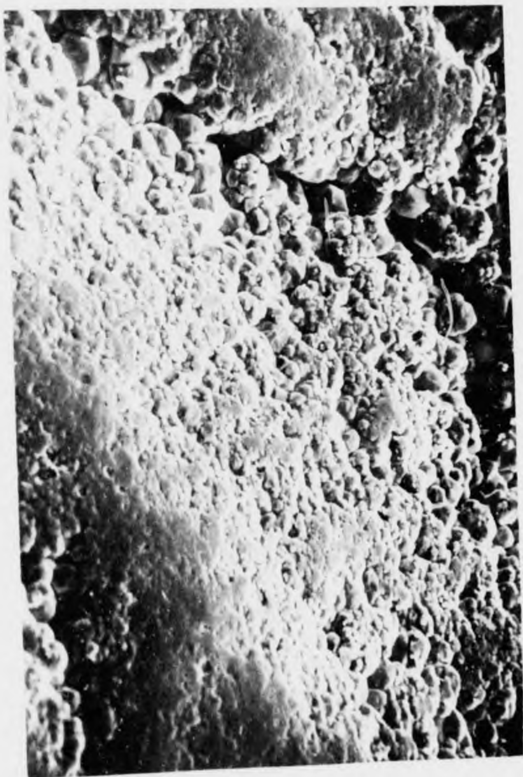
Scanning electron micrograph of the surface of a specimen, showing a dense, granular texture. (Mag. 1200X)
