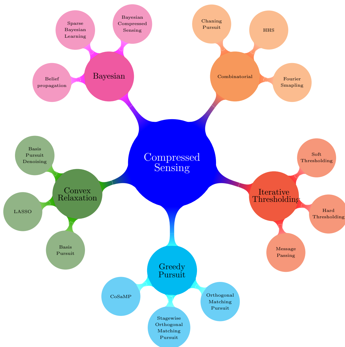
Figure 3.1: Classification of compressed sensing algorithms.
