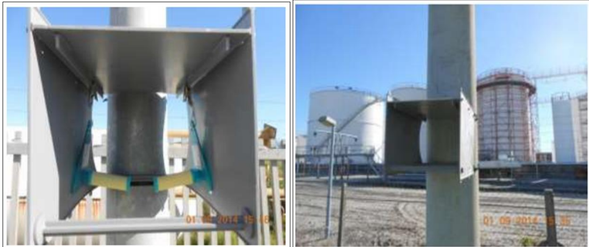
Figure 3.3: Radiello Passive samplers on the mounted support plate placed inside a mountable shelter on site.
