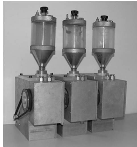
Figure H9: The flexible numerical control powder feeder unit, (a) Schematic drawing and (b) photograph (Zou et al., 2008)
