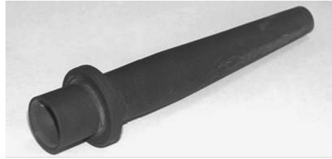
Figure 4.38: An axisymmetric supersonic CD nozzle unit (Papyrin et al., 2007)
