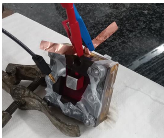
Figure 25: a) The assembled zinc-air battery. b) Power profiles of the standard 20% Pt/C + \text{IrO}_2 cathode and the 20% HESO/C cathode, with and without an applied field
