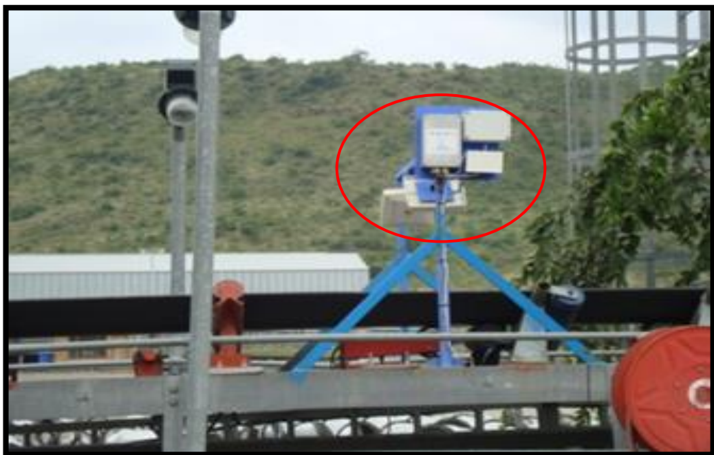
Figure 33: Tag Reader on Conveyor Belt System (Bruwer, 2021)
