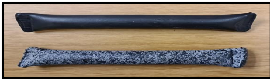
Figure 30: Radio Frequency Identification Device Tags – Top Tag for UG2 & Bottom Tag for Waste (Bruwer, 2021)
