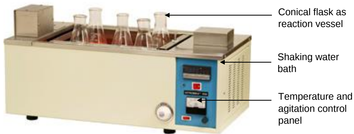
Figure 6.1: Organic/aqueous dispersion experimental setup with conical flasks
