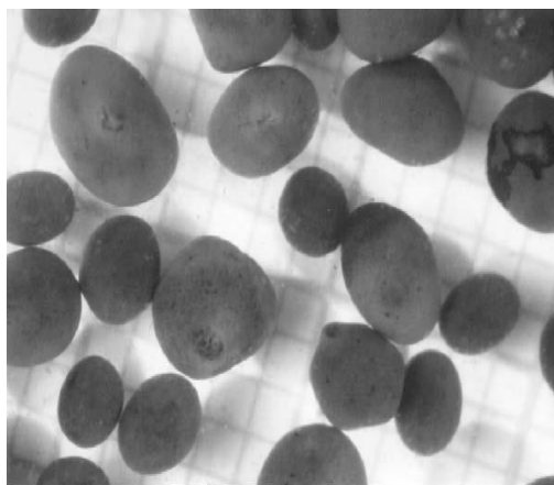
Figure 2.10: Typical example of granules from a UASB anaerobic reactor (Hulshoff et al., 2004)
