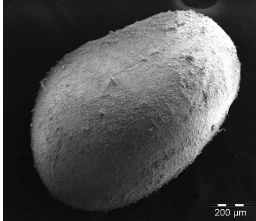
Figure 5.16: The SEM image of a granule that has been treating wastewater for 38 days (LS IC-AD Run 1)
