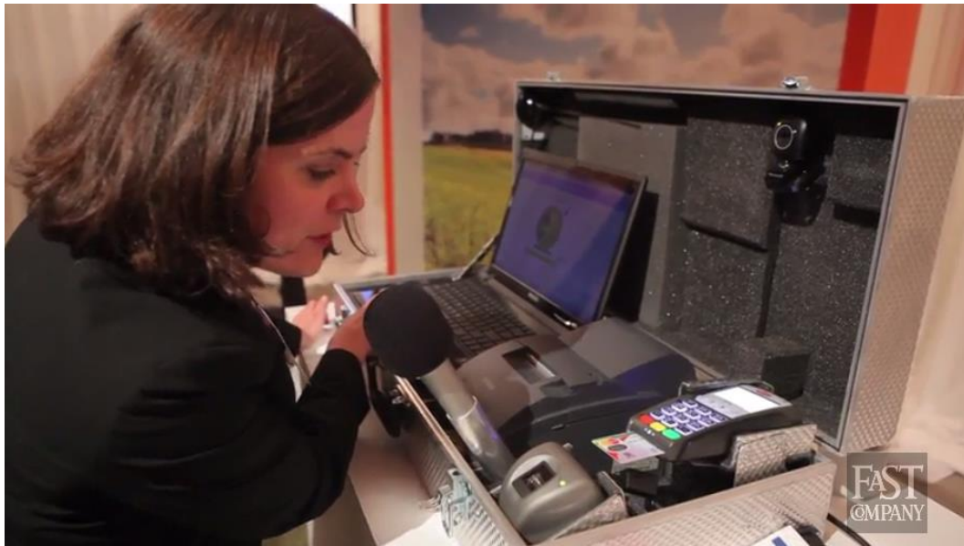
Figure 4 Close-up view of MasterCard demonstrational enrolment and payment kit featuring laptop, printer, microphone, camera, card reader, and fingerprint reader enclosed in metallic case
