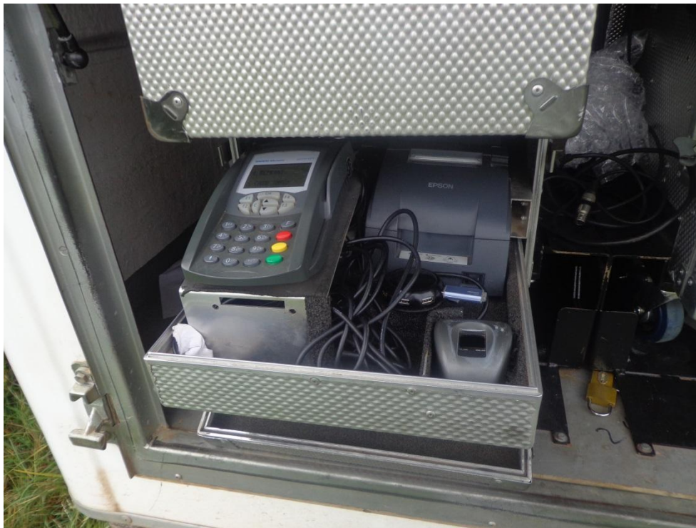
Figure 5 Payment kit with standalone fingerprint reader mounted on a vehicle
