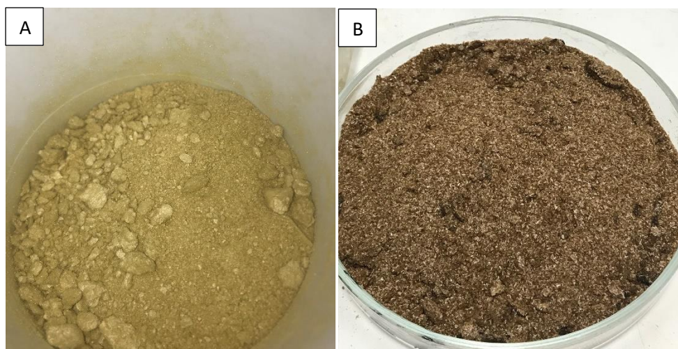
Figure 3.2. Shows imidate derivate products isolated through filtration. (A) shows pale-yellow solid MADI, (B) shows brown-crystalline solid EADI.
