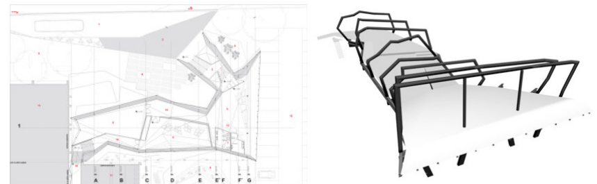
Figure 3.62: Nestle Chocolate Museum - free form portal frame with variable shapes, sizes and spans (Karmatrendz, 2009; Fairs, 2007).
