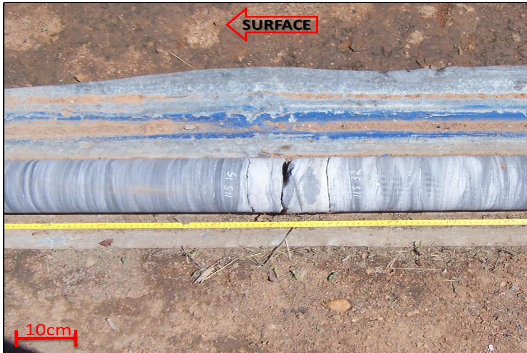
Figure 3.10: Cross-laminated sandstone sub-lithofacies (Sr) showing flaser and wavy stratification across the sandstone unit.
