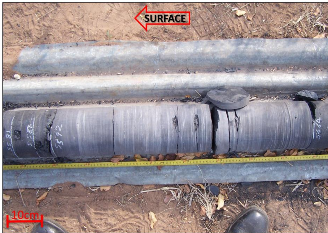
Figure 3.15: Lenticular laminated siltstone (Fsn) sub-lithofacies comprising fine to medium-grained sandstone laminae throughout the unit.
