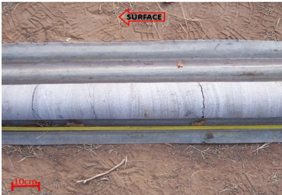
Figure 3.9: Planar cross-bedded sandstone (Sp) sub-lithofacies, with planar-bedded mica bands across the unit.
