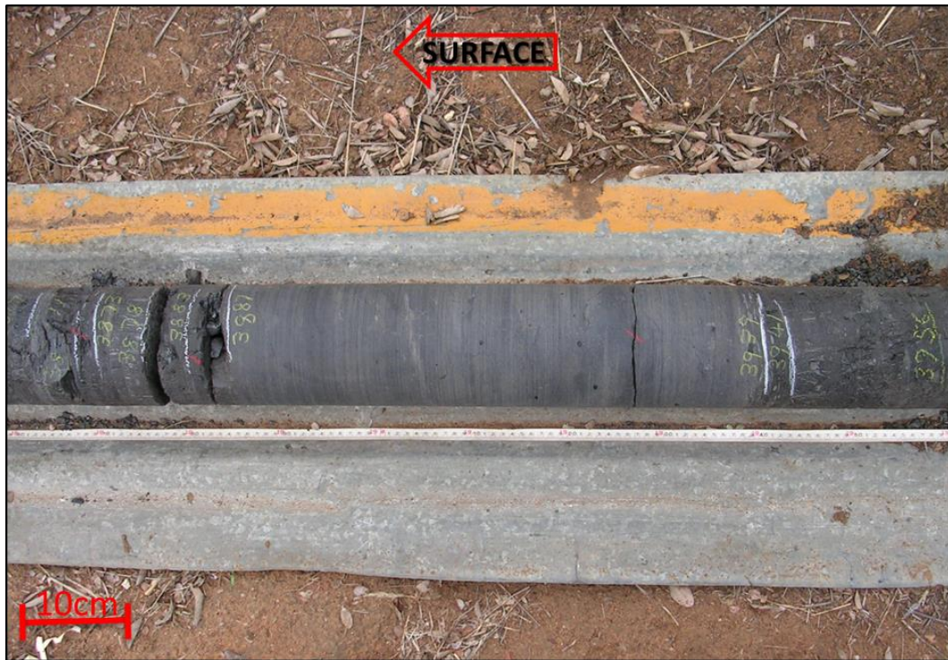
Figure 3.13: Horizontally laminated mudstone (Fh) sub-lithofacies capped sharply by coal.
