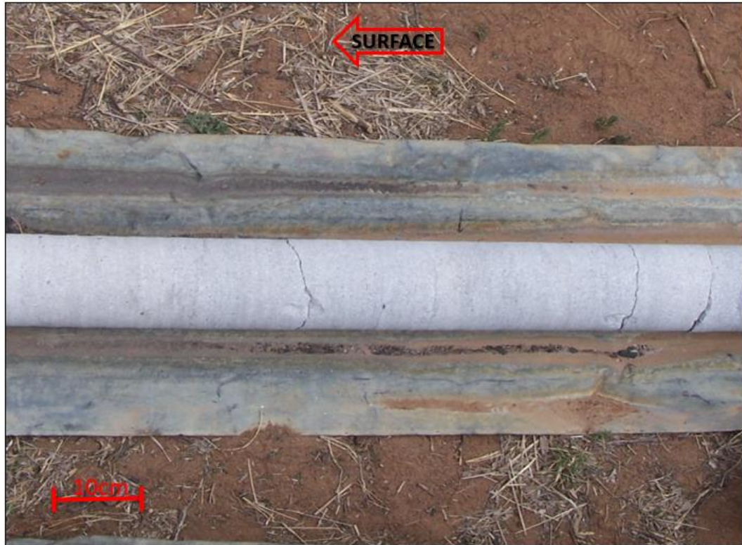
Figure 3.8: Massive sandstone (Sm) sub-lithofacies comprise coarse-grained, highly competent, and tightly packed quartz grains.
