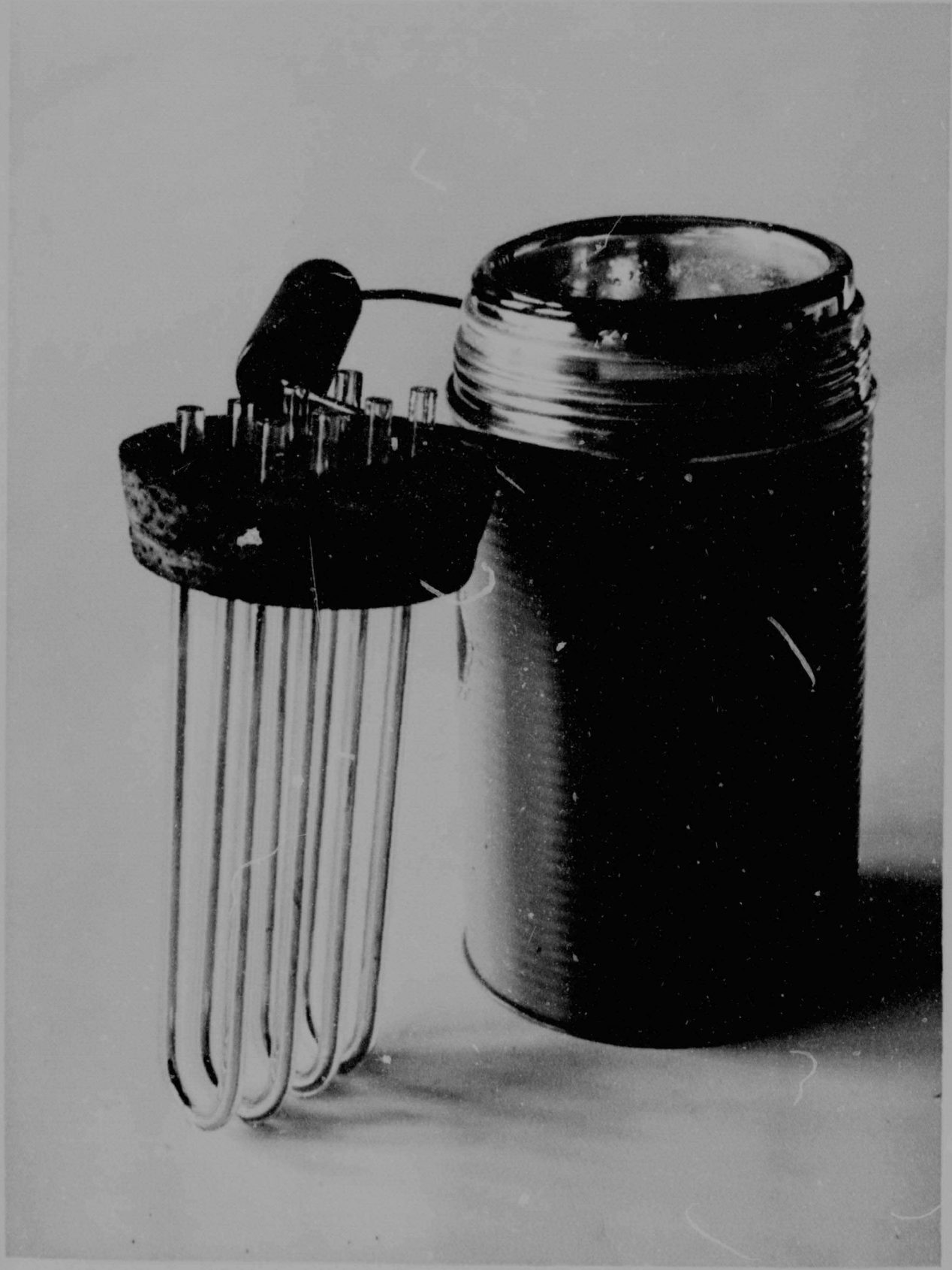
FIGURE II, 7. WIDE NECKED THERMOS FLASK, SHOWING MERCURY-FILLED U-TUBES IN CORK TOP.
