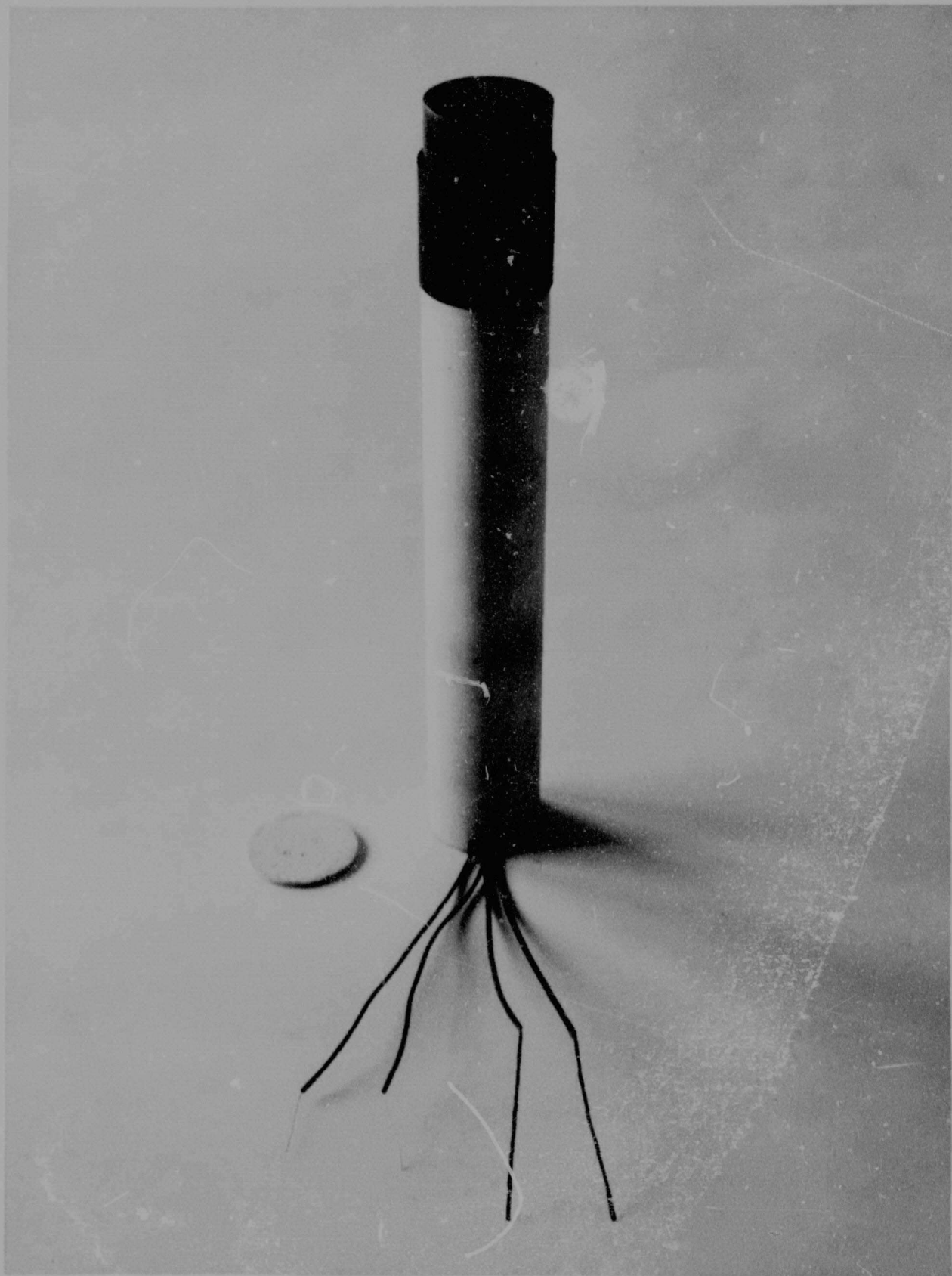
FIGURE II, 5. VERTICAL FURNACE SAMPLE HOLDER COMPONENTS ASSEMBLED
