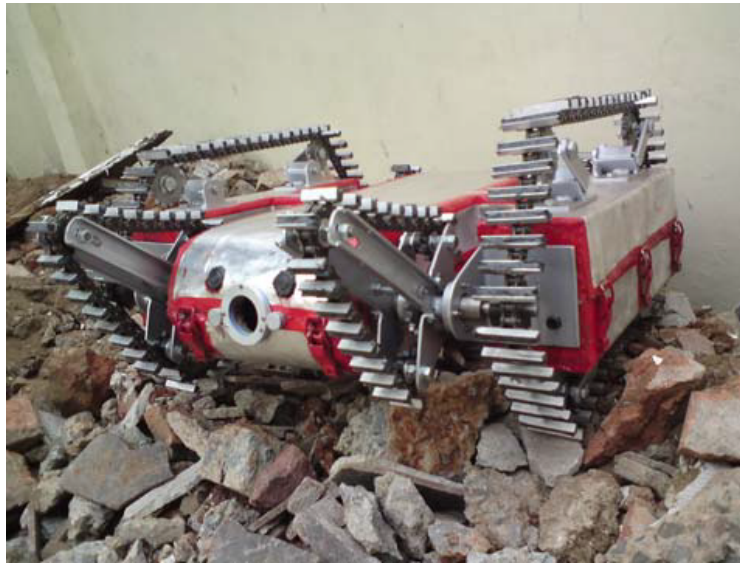
Figure 2.1: The CAESAR tracked-robot, which provides thermal imaging and CO, CO 2 , H 2 S, methane and oxygen sensors for disaster scenarios, amongst its many other sensory and communication technologies.
