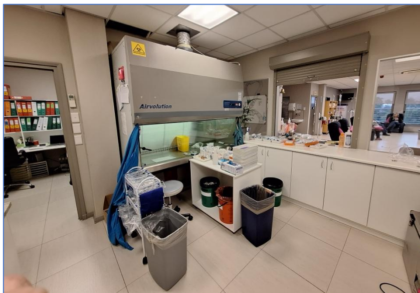
Figure 1. A Containment-primary engineering control (C-PEC), otherwise known as a vertical airflow HEPA filtration laminar flow unit or biological safety cabinet (BSC) where antineoplastic drugs are typically compounded
