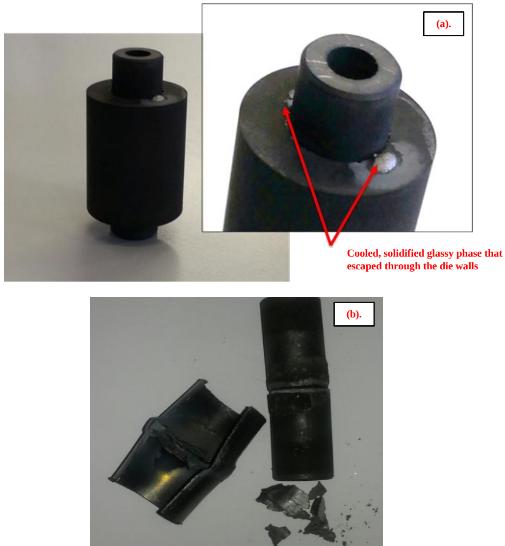
Figure 27: An image of the graphite dies ruptured during a sintering process
