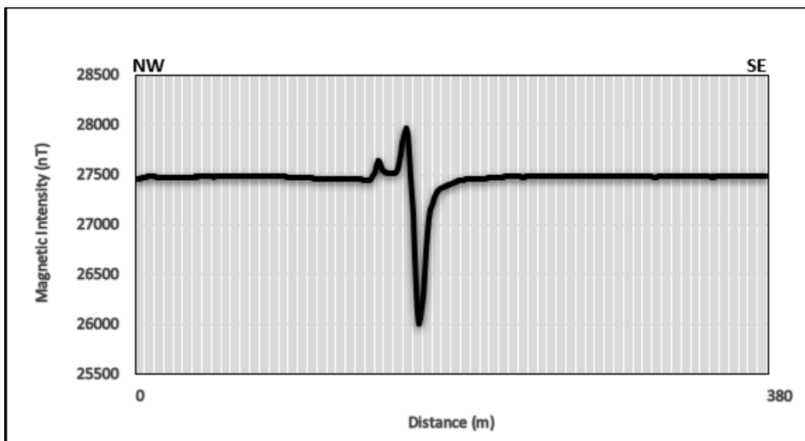
Figure 25: The magnetic intensity data was recorded along lines 4 (L_4) with the traverses in the NW-SE directions with the linear structure positions indicated.
