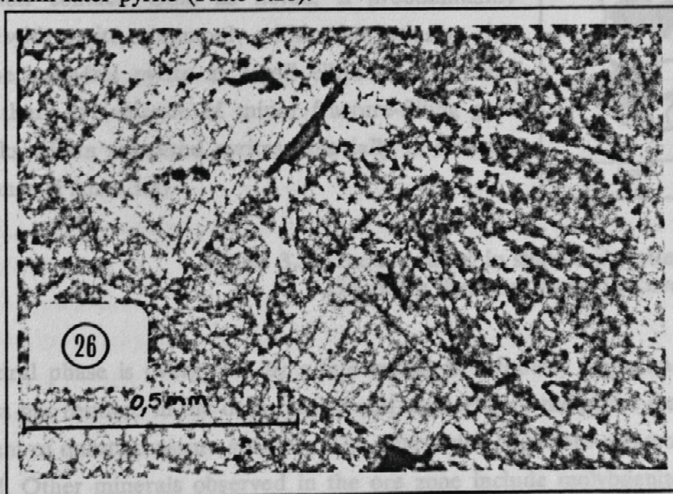
Plate 3.26. Euhedral, digenetic / metamorphic pyrite occurring within later auriferous pyrite. Sample stained with acidified \text{KMnO}_4 . Discovery Shaft 11-level
