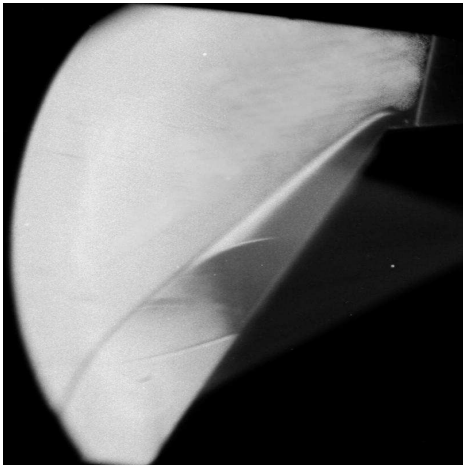
Figure 192: Schlieren images for triangular valley, \theta_w = 70^\circ , \theta_v = 15^\circ , at time delay 1600\mu\text{s} , 1625\mu\text{s} , 1675\mu\text{s} , and 1700\mu\text{s} respectively.
