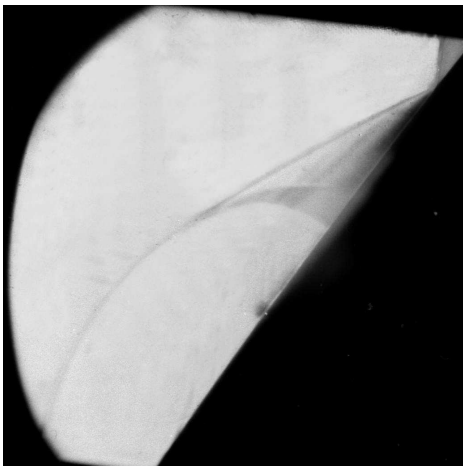
Figure 248: Schlieren images for parabolic valley, a = 0.055 , at time delay 1650\mu\text{s} , 1675\mu\text{s} , 1700\mu\text{s} , 1725\mu\text{s} , and 1750\mu\text{s} respectively.
