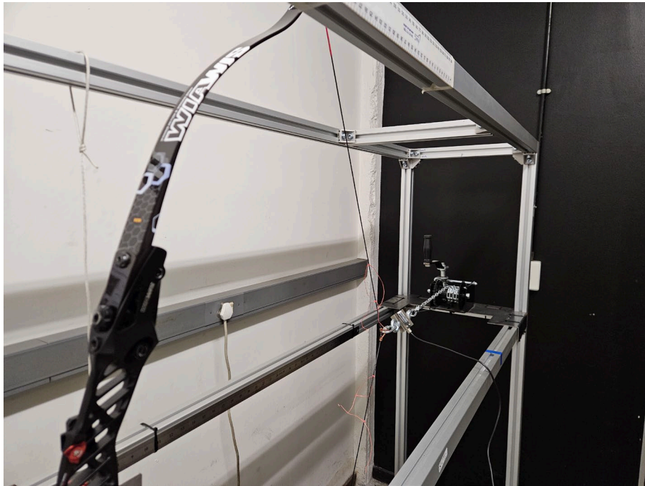
Figure 24 - Compliance test set-up.
