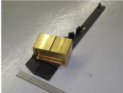
Figure 3.5: The (p,t) beamstop. Note that it consists of two separate brass blocks, each with dimensions 70 mm (deep) x 55.5 mm (wide) x 55 mm (high). These dimensions includes the lip, which is 5 mm wide and 10 mm deep.
