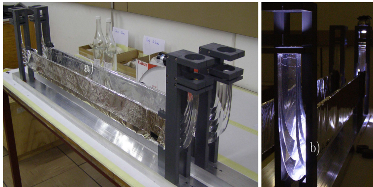
Figure 3.8: Plastic scintillator paddles of the K600 focal plane detector system [24].
