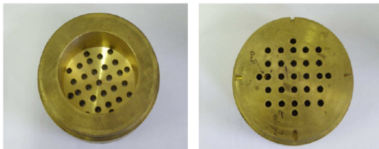
Figure 4.9: A picture of the pepper-pot collimator for the small angle mode. The back of the collimator, i.e. the side facing the K600, is 862.27 mm from the target. The first hole from the middle on either axis is positioned at 0.63^\circ , the second hole at 1.26^\circ and the third hole at 1.79^\circ , spanning approximately 4.64 mrad [40].
