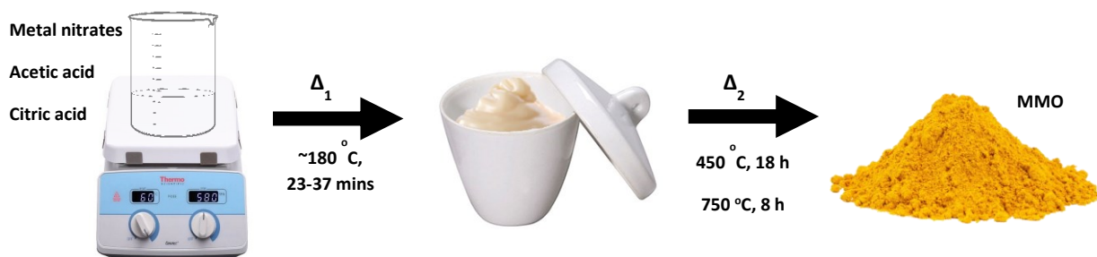
Figure 2.23. Schematic illustrating the citrate sol-gel method utilized to synthesize the materials presented in this thesis.
