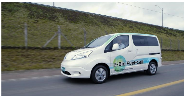
Figure 1.6. The result of the Nissan Intelligent Power program - the world's first car powered by SOFC technology. 63
