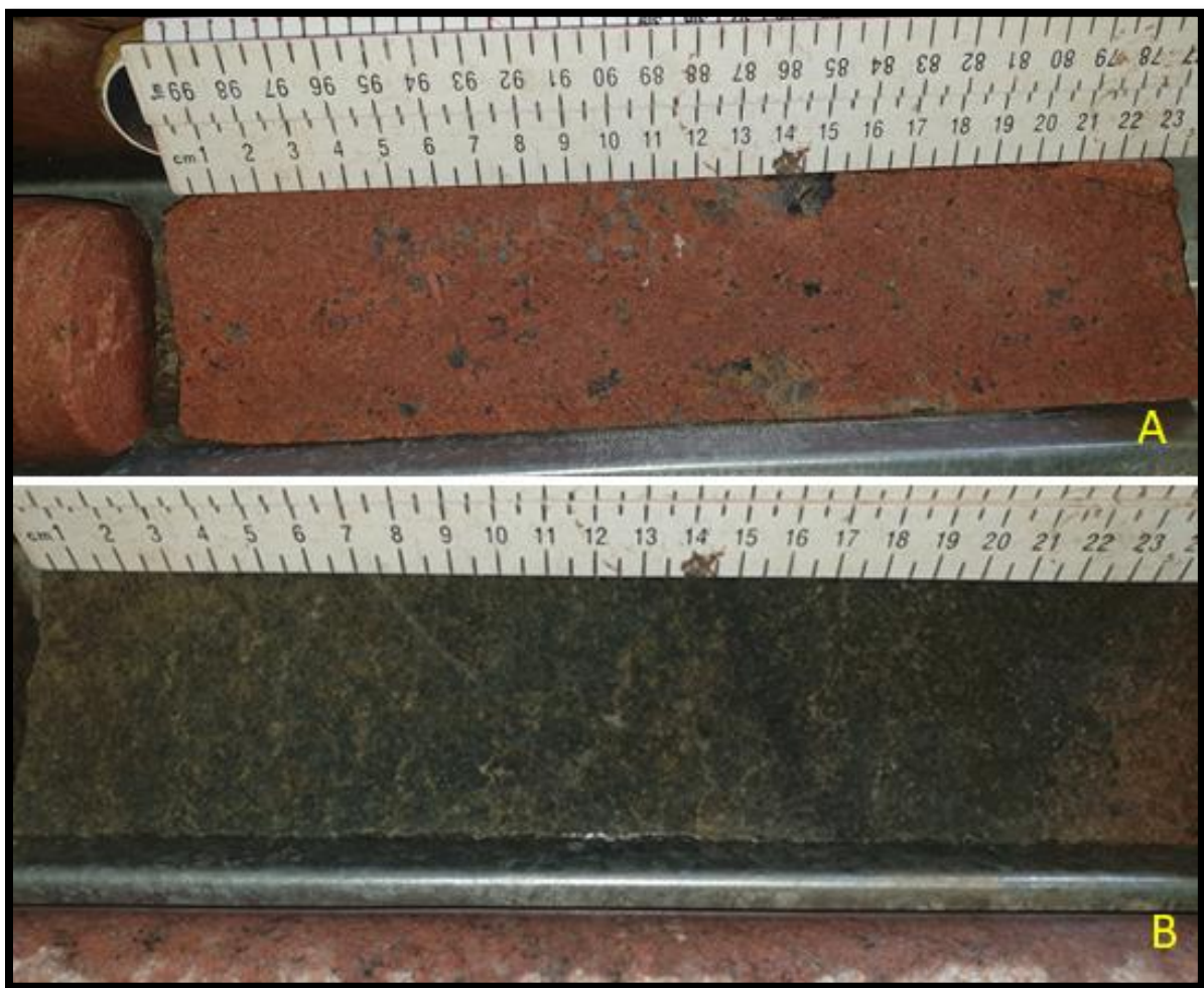
Figure 5.14. Photographs from 648 KS/1 core of aplitic granite. A: Typical porphyritic aplitic granite. B: Altered aplitic granite (possibly albitized). The albitized portion is devoid of phenocrysts (core depth between ca. 116.00 and 120.00 m).
