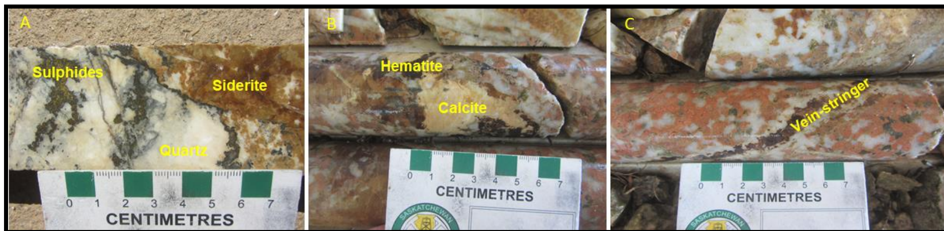
Figure 5.6: Photographs from BHDD 003 core showing the typical mineralogy of veins crosscutting the Nebo granite. A: siderite-calcite-quartz-sulphides vein crosscutting the Nebo granite. B and C: Relatively small hematite veins and calcite veins and hematite vein-stringers often crosscut the Nebo granite core (Images represent depths between ca.163.00 and 194.00 m).
