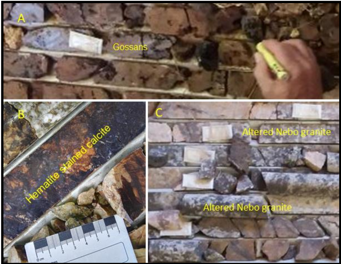
Figure 5.3: Photographs from BHDD 003 core showing gossan-stained Nebo granite and gossans. A: botryoidal hematite and network of weathered acicular-goethite prisms (image taken between 17.28 and 19.60 m depth). B: Hematite stained calcite vein (Image taken between 19.60- 30.31 m) and gossans topping the BHDD 003 core.
