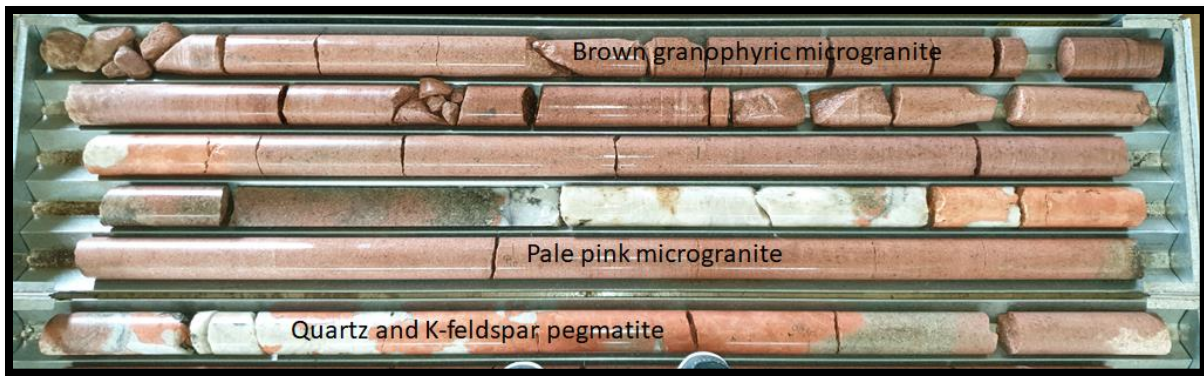
Figure 5.15: Photograph from 648 KS/1 core showing brown granophyric microgranite (top) grading into the pink variety (bottom), both microgranites are crosscut by large pegmatite pockets. Tray size =1.5m (core depth between ca. 53.00 and 60.50 m).
