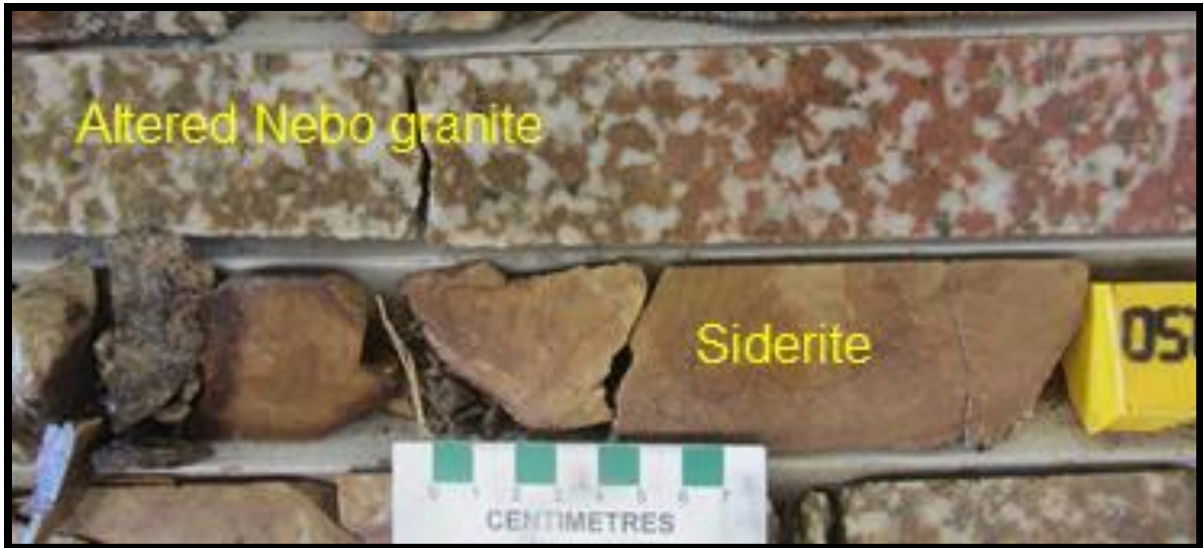
Figure 5.5: Photograph of BHDD 003 core showing the transition of granite to altered granite. The altered granite often encloses veins (core depth between ca. 116.00 and 120.00 m).
