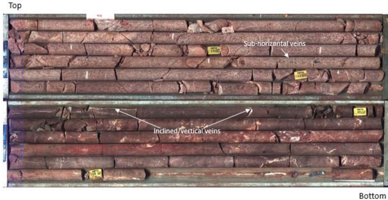
Figure 4.13. Drillcore images show changes in frequency and orientation of veins within the M4 drillcore. The top drillcore box shows monzonitic gneiss (110.08 – 119.39 m depth) displaying subhorizontal calcite veins. The bottom drillcore box shows metadolerite (194.46 – 202.6 m depth) and suevite displaying subvertical veins of zeolite veins (annotated with arrows) and pre-impact quartz veins. The drillcore width is 4.5 cm.
