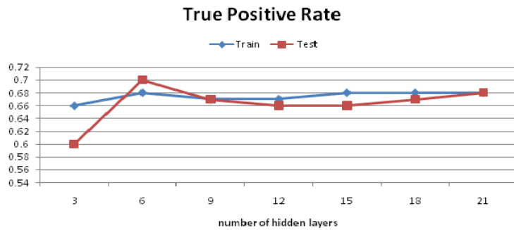
Figure 23: Sensitivity for a change in the number of hidden units in ANN model
