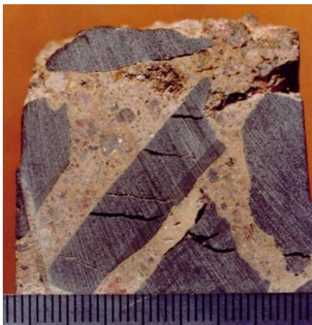
Figure 2: The enemy without – Damage to the near surface zone of concrete on which sodium sulphate was regularly spilt in a production process (the scale at the bottom of the picture is in mm).
