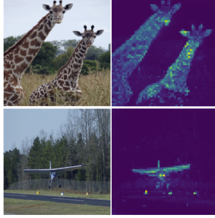
Figure 3.5: Attention maps obtained from the final layer of a Vision Transformer (ViT) trained using the self-supervised learning method DINO [Caron et al. 2021].
