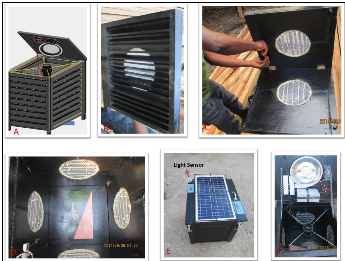
Figure 6: Pictorial representation of the odour-baited mosquito landing box (A) fitted with electrocuting grids (B, C and D) and an automated on/off light sensitive switch (E) that activates the device at dusk and stops it at dawn. The entire electric system and the odour-dispensing system are powered by a 12-volt solar rechargeable battery (F) , allowing for a passive but effective mosquito control and surveillance system.
