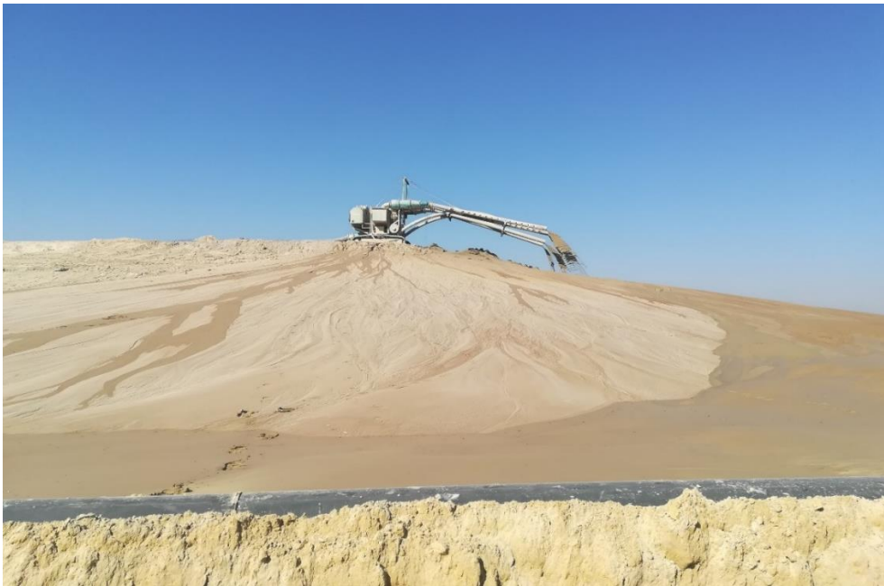
Figure 3.4. A cyclone depositing new tailings at Site B.
