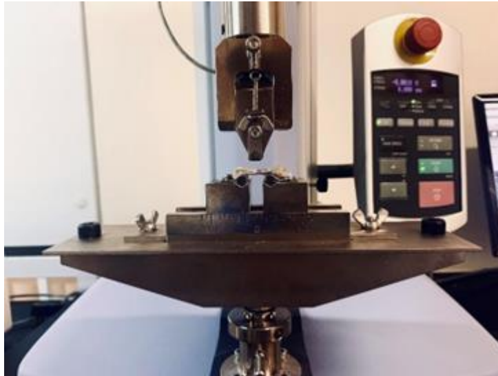
Figure 2.1: Three-point bending test using the Shimadzu 3-point bending machine (Figure provided by R.Rakgoathe)
