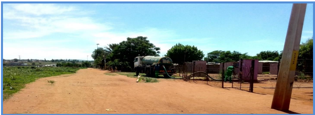
Figure 4. 12: A contracted ‘honey sucker’ desludging a VIP toilet system. Source: Author’s 2020
