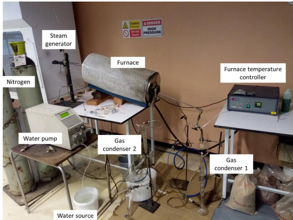
Figure 3.7: The pyro-gasification rig.
