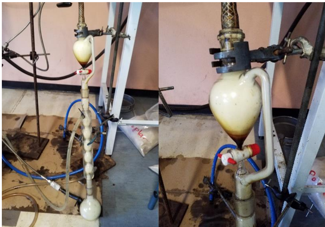
Figure 6.21: Bio-oil deposition through condensation of heavy pyrolysis gases
