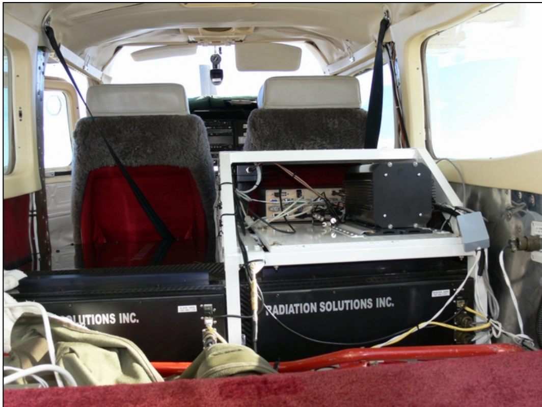
Figure 4-1 Two RS-500 detector packs fitted in airplane (Picture courtesy of Radiation Solutions Inc.).
