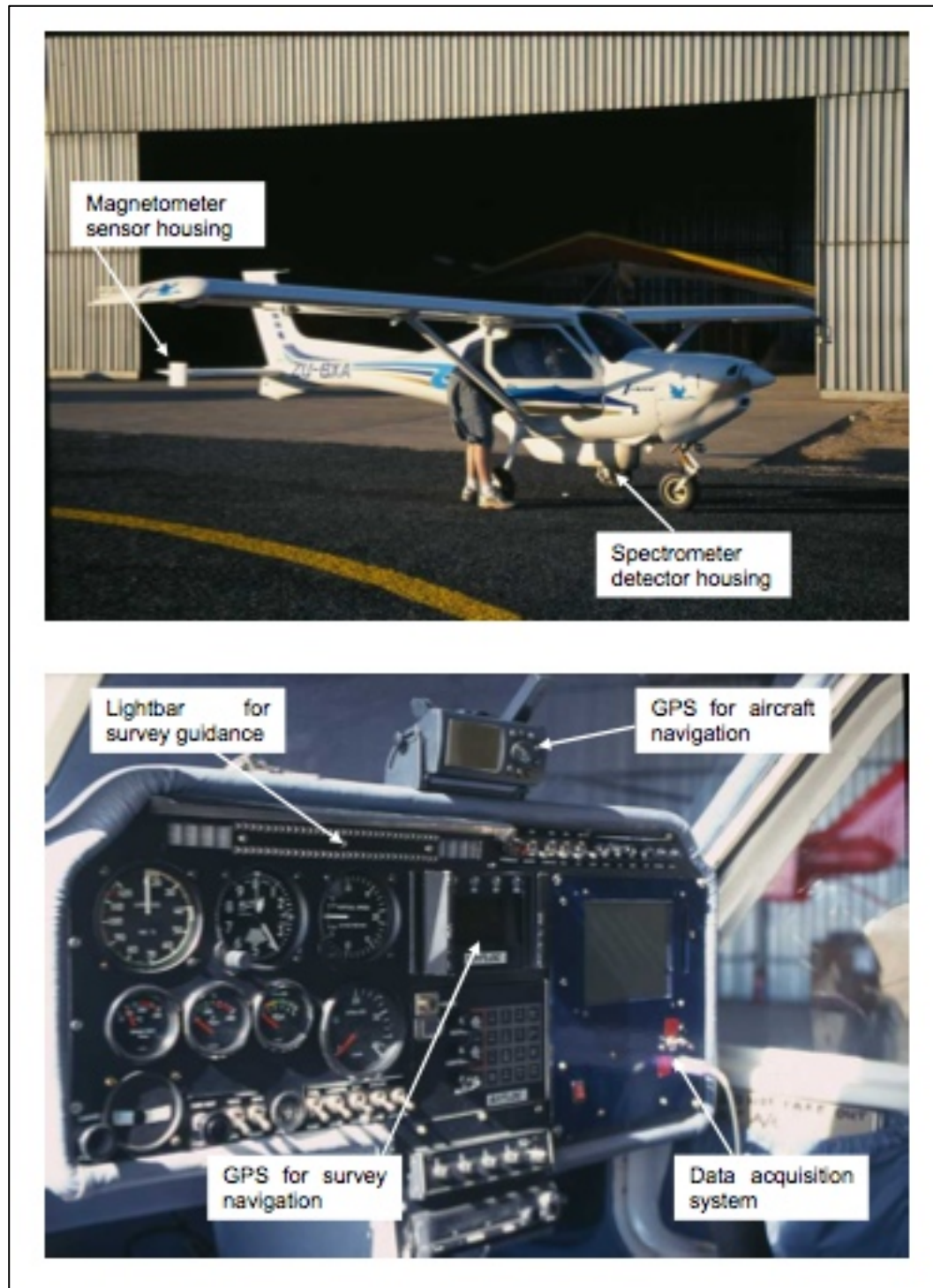
Figure 4-3 The airplane (Jabiru) used for the survey work (photo courtesy of Council for Geosciences), note the detector housing under slung and the electronics in the cockpit.
