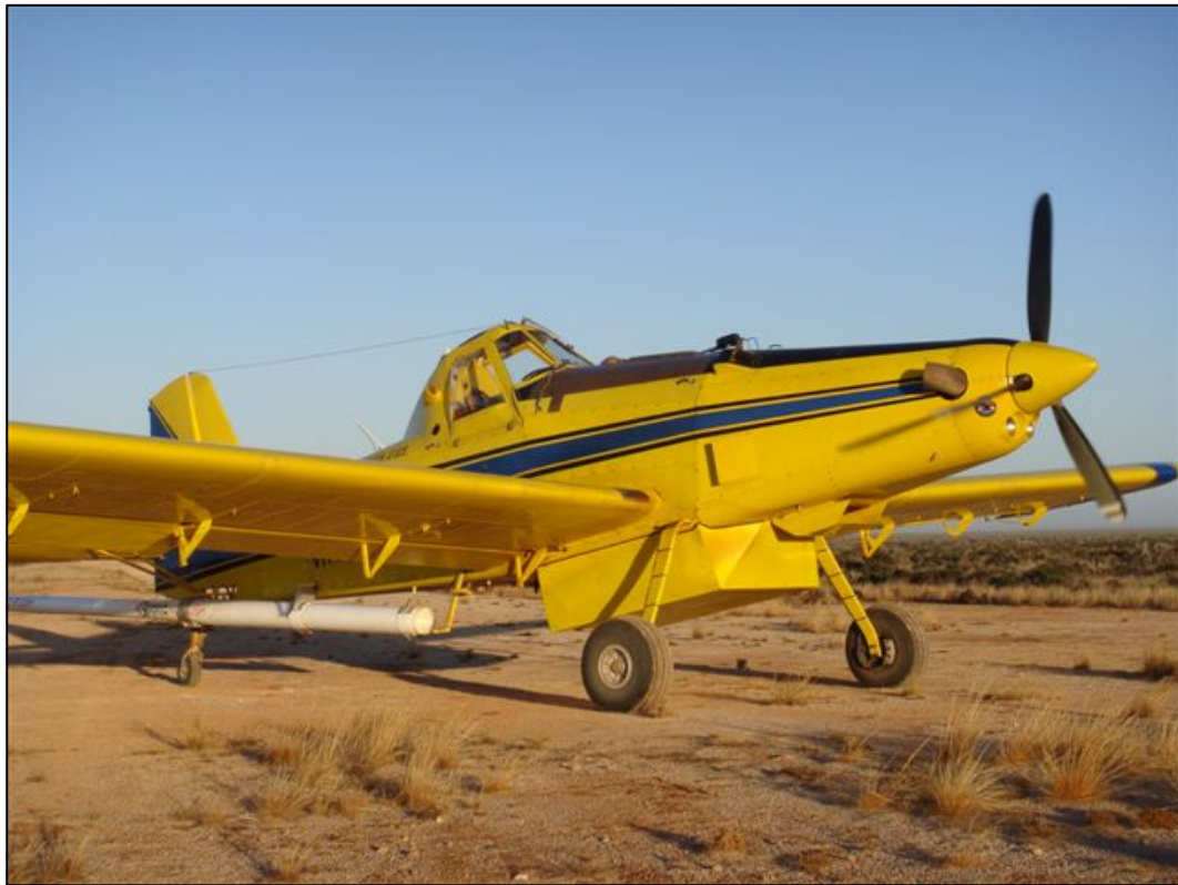
Figure 4-4 Air Tractor Data Boss 502 'Data Boss' with under-slung detectors
