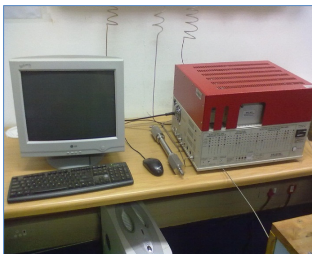
Figure 3.9: GC connected to online PC
