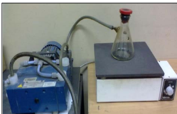
Figure 3.4: Degassing Set-up: vacuum pump, hot-plate and glassware
