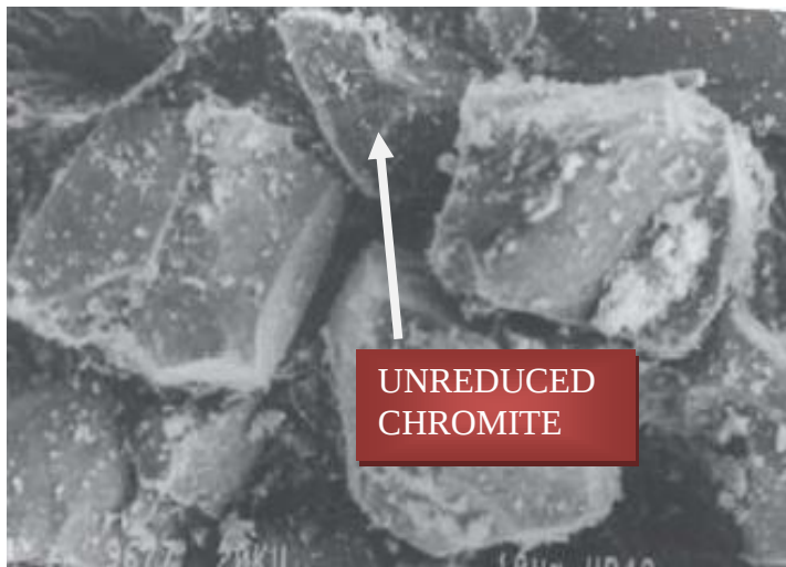
Figure 4.40. Scanning electron microscopic image of unreduced chromite
