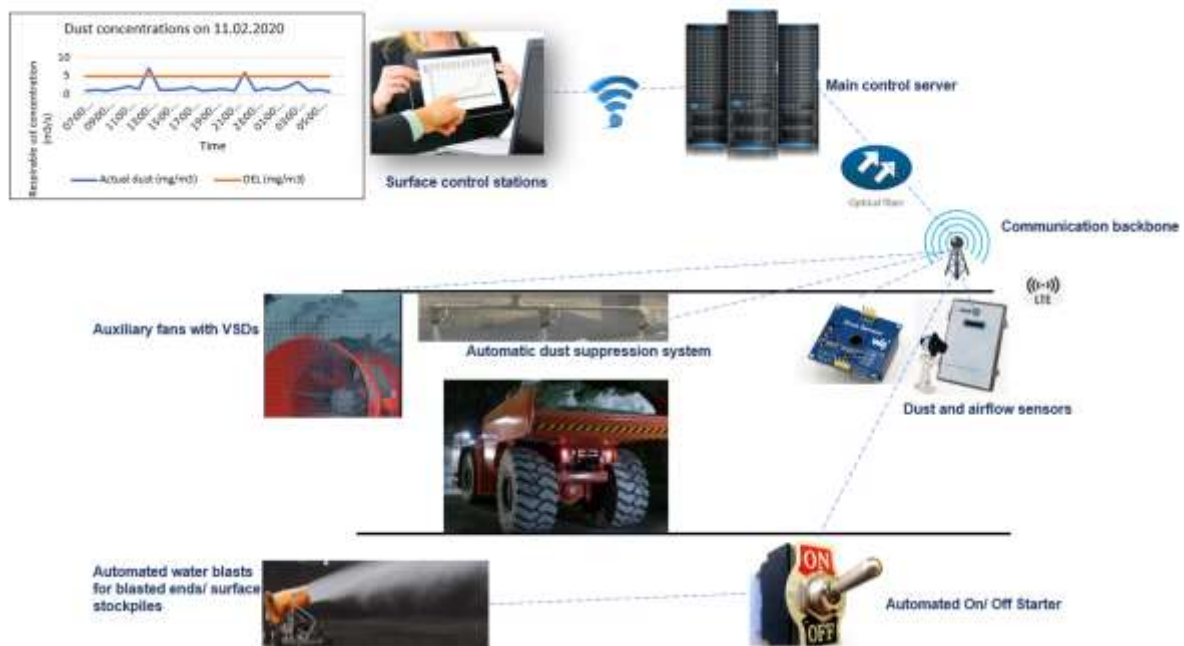
Figure 5.20: Underground dust management system
