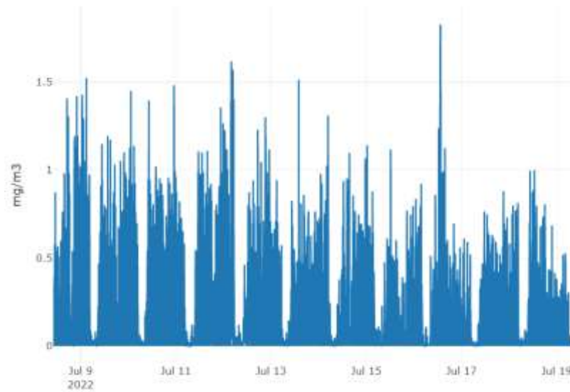
Figure 2.11: Real-time respirable dust concentration in the research area (extracted from research - Trolex system)
