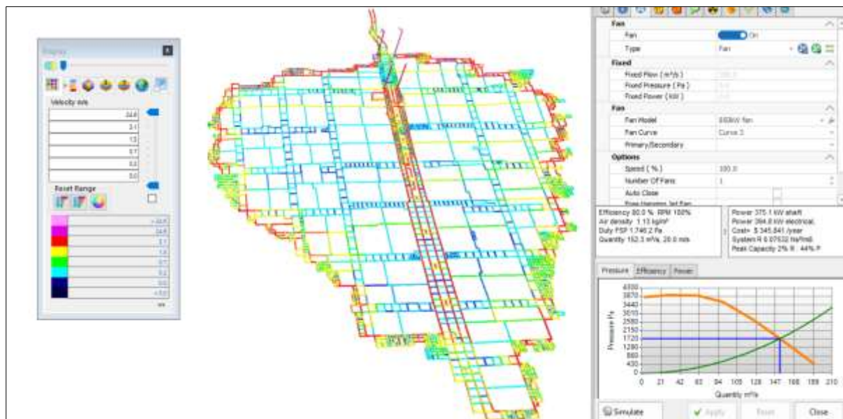
Figure 3.16: Power consumption for main surface fans
