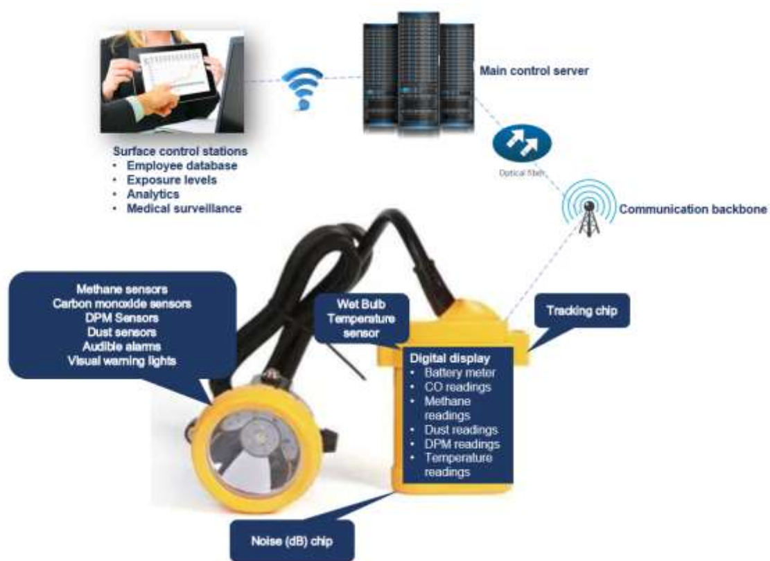
Figure 5.21: Underground smart cap lamp
