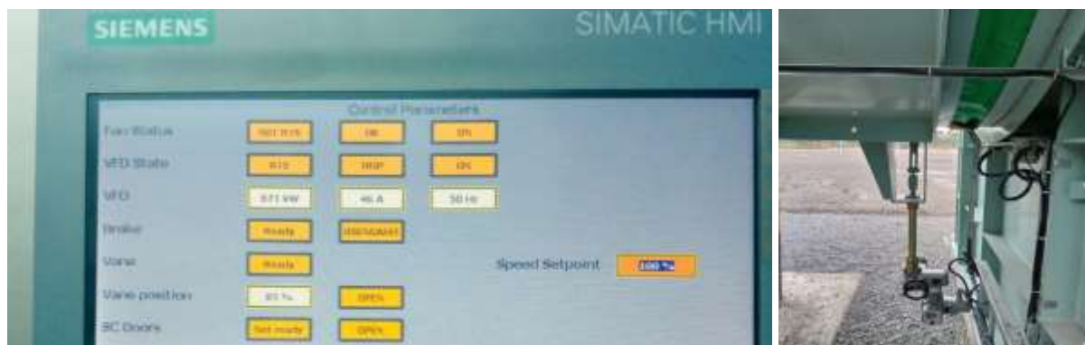
Figure 5.7: Airflow regulation by RVC
