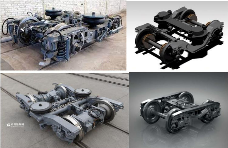
Figure 15. top left: locomotive bogie (Allert, 2013), Top right: trailer coach bogie (Shubhamkar, 2020), Bottom left: motorized coach bogie (CRRC, 2016), Bottom right: wagon bogie (Tatravagónka, 2016)
