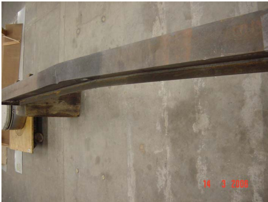
Figure 4.6a – Specimen at failure (out-of-plane global buckling)
