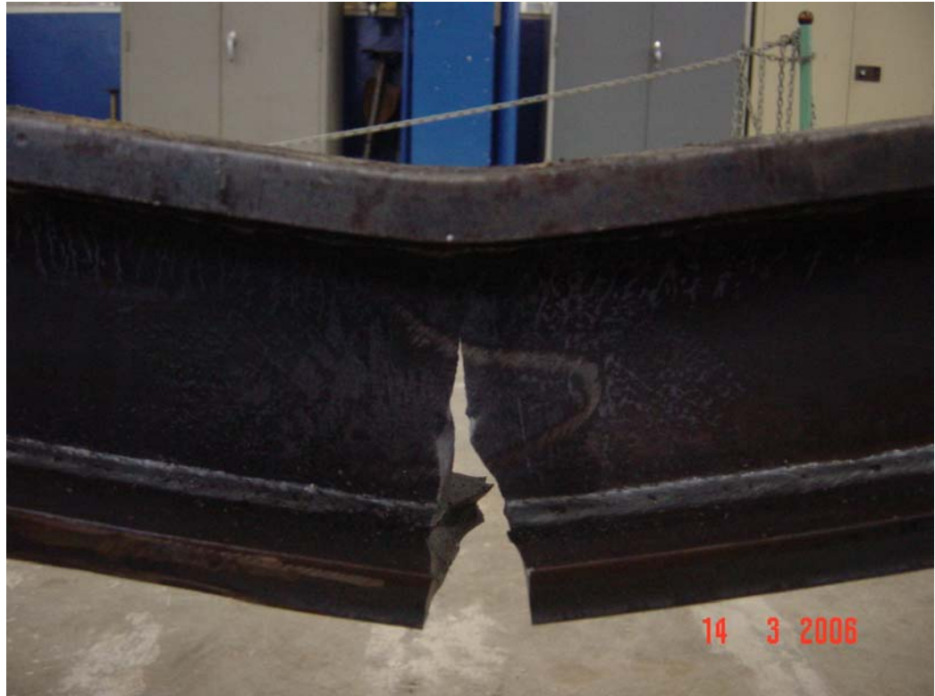
Figure 4.14b – Specimen at failure
