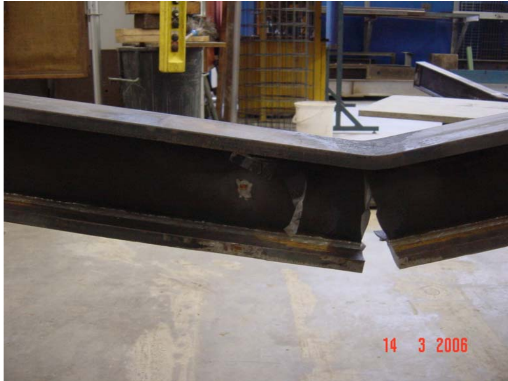
Figure 4.10b – Specimen at failure
