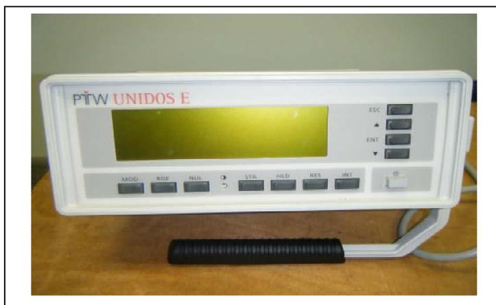
**Figure 3.4:** The PTW T10008 Unidose E Electrometer
